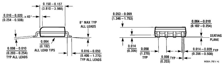
**8-Lead Small Outline Integrated Circuit (SOIC), JEDEC MS-012, 0.150" Narrow
