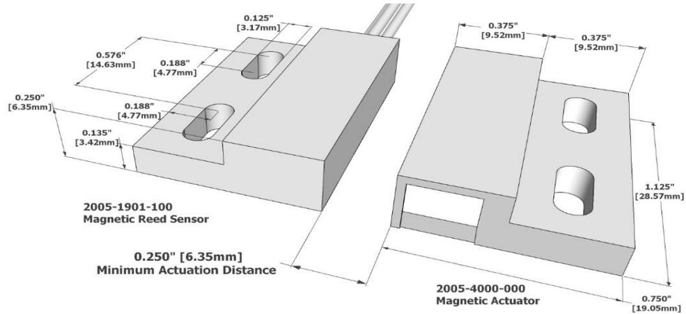
All measurements are in Inches [millimeters]
