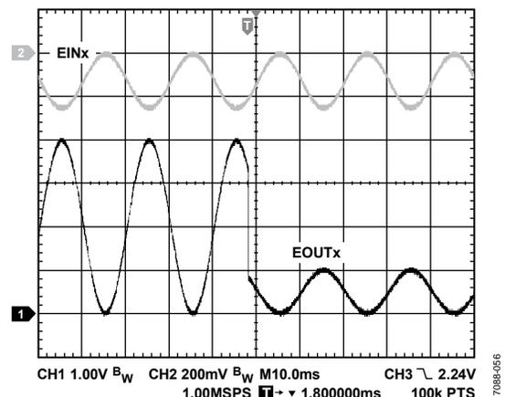
Figure 57. PGA Gain Switching from Gain = 16 to Gain = 4
