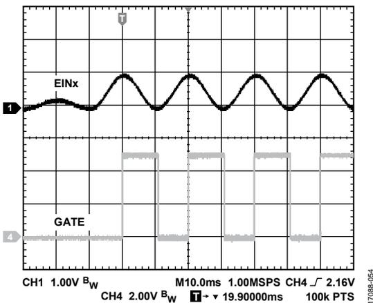
Figure 55. Analog Trip Threshold Triggered, VCOM = RCOM = 0V
