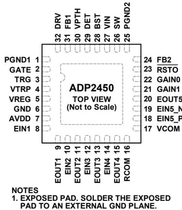
Figure 3. 32-Lead LFCSP Package Pin Configuration (Top View)
