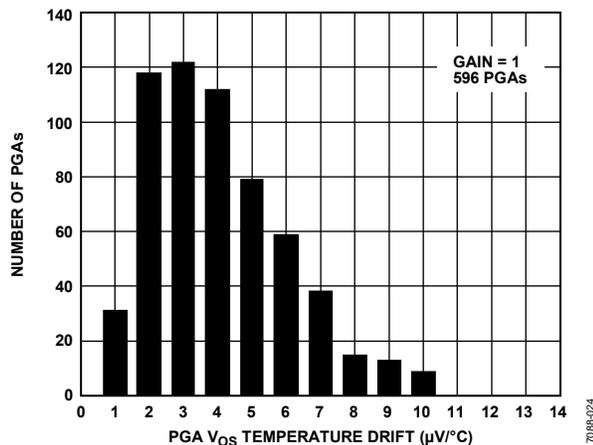
Figure 25. PGA Input Offset Voltage Drift Distribution, Gain = 1
