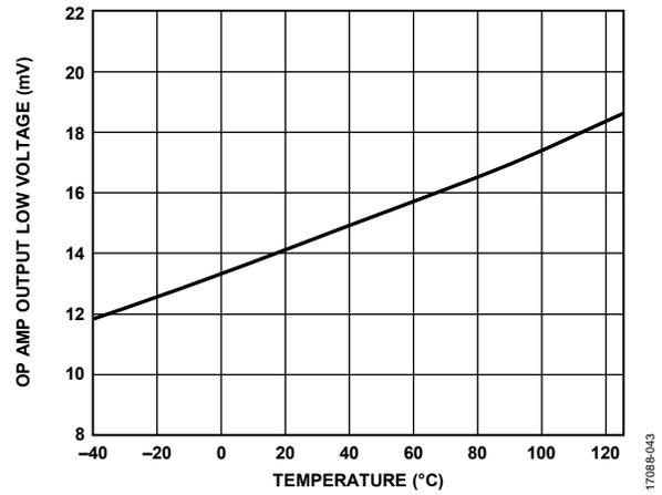
Figure 44. Op Amp Output Low Voltage vs. Temperature
