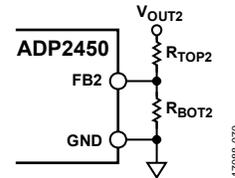
Figure 71. Buck Regulator Adjustable Output Voltage Setting
