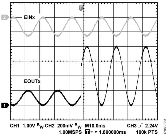
Figure 54. PGA Gain Switching from Gain = 4 to Gain = 16
