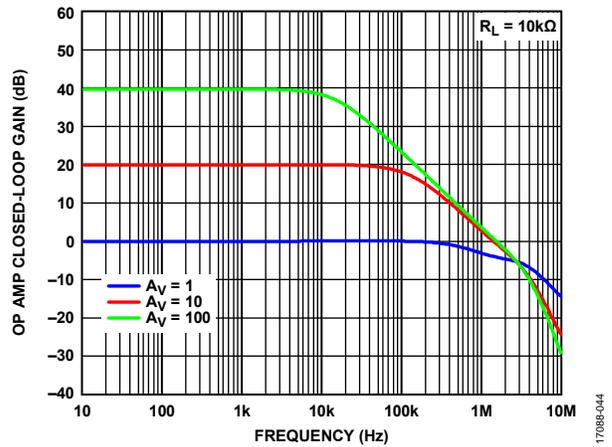
Figure 45. Op Amp Close-Loop Gain vs. Frequency
