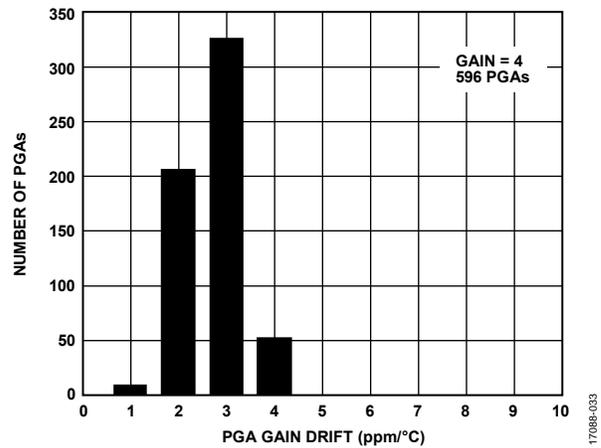
Figure 34. PGA Gain Drift Distribution, Gain = 4
