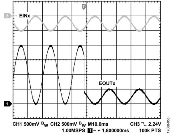
Figure 56. PGA Gain Switching from Gain = 4 to Gain = 1
