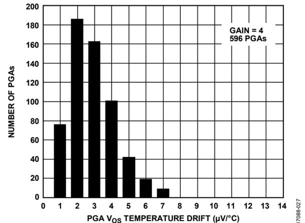
Figure 28. PGA Input Offset Voltage Drift Distribution, Gain = 4
