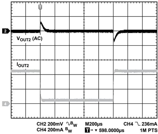
Figure 61. Buck Regulator Load Transient (50 mA to 450 mA)
