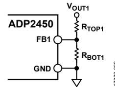
Figure 70. Boost Shunt Controller Output Voltage Setting
