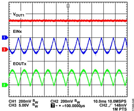
Figure 49. PGA Working Waveform, Gain = 1
