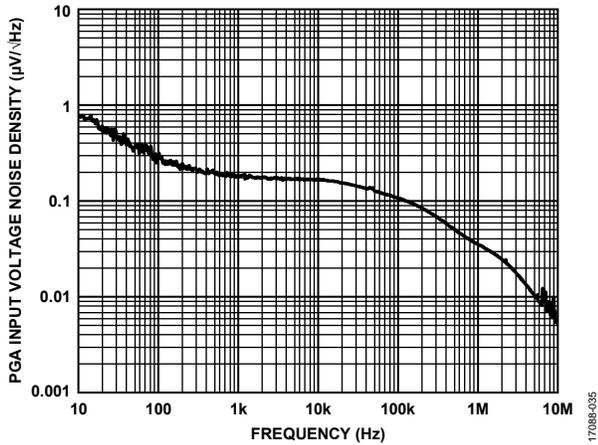
Figure 36. PGA Input Voltage Noise Density vs. Frequency
