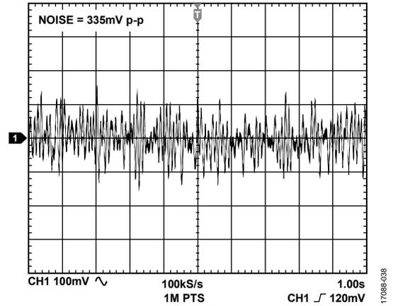
Figure 39. PGA 0.1 Hz to 10 Hz Noise, Amplification = 10,000x
