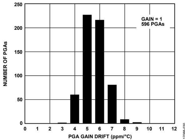
Figure 31. PGA Gain Drift Distribution, Gain = 1
