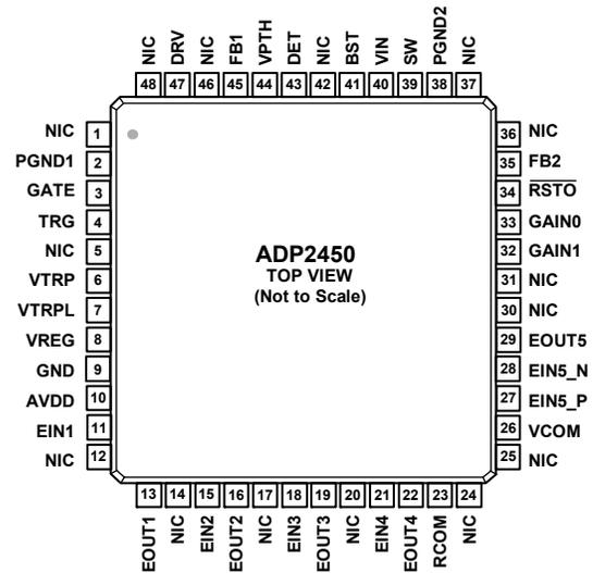
Figure 4. 48-Lead LQFP Package Pin Configuration (Top View)
