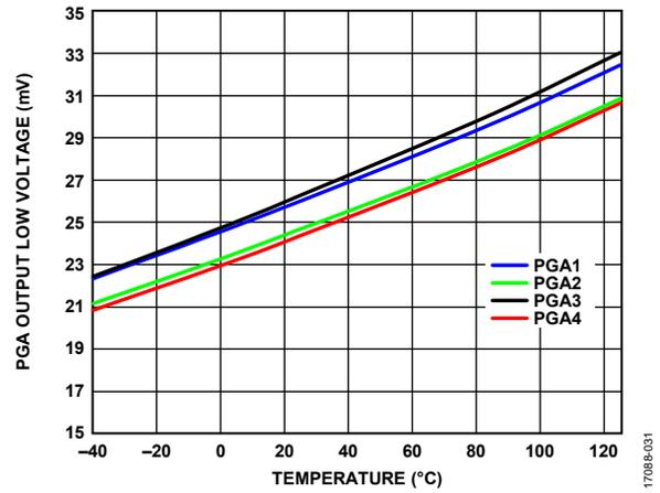
Figure 32. PGA Output Low Voltage vs. Temperature
