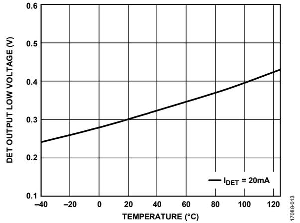
Figure 14. DET Output Low Voltage vs. Temperature
