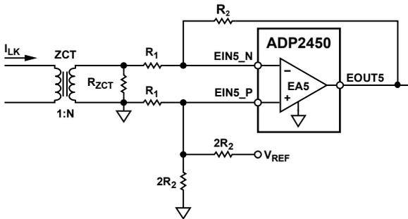
Figure 67. Typical Configuration for Leakage Current Detection
