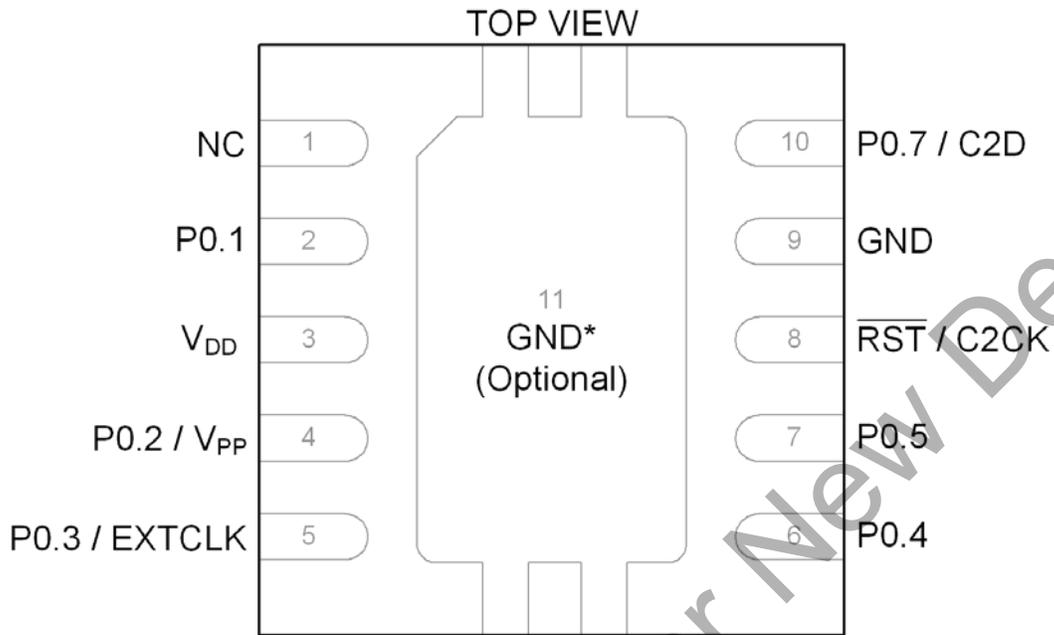
Figure 3.3. C8051T606-GM QFN11 Pinout Diagram (Top View)
