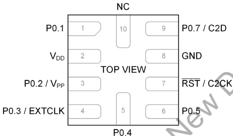
Figure 3.5. C8051T606-ZM QFN10 Pinout Diagram (Top View)
