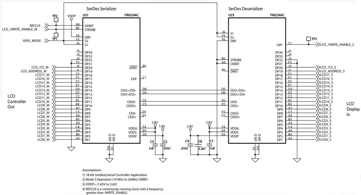
Figure 6. FIN224AC Microcontroller
