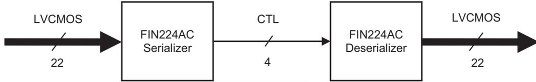
Figure 1. Conceptual Diagram
