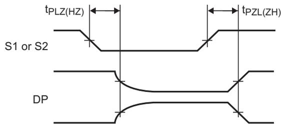
**Note:** If S1(2) transitioning then S2(1) must = 0 for test to be valid
