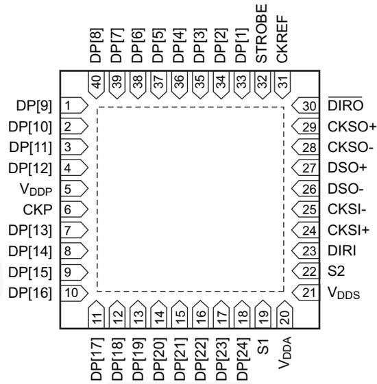
Figure 3. Terminal Assignments for MLP (Top View)
