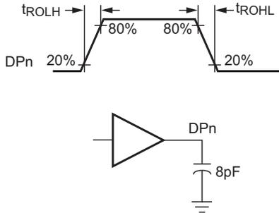
**Figure 7. LVC MOS Output Load and Transition Times**
