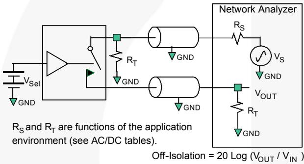
$R_S$  and  $R_T$  are functions of the application environment (see AC/DC tables).
