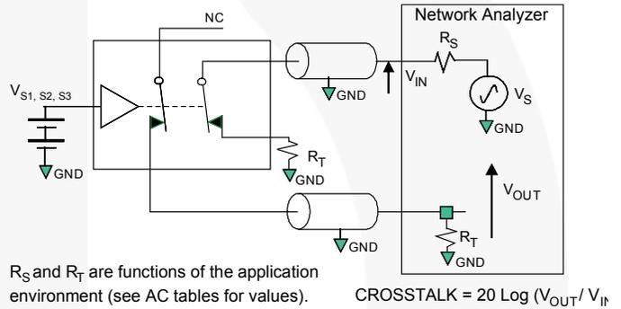
$R_S$  and  $R_T$  are functions of the application environment (see AC tables for values).
