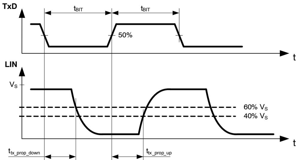
Figure 13. Definition of LIN Transmitter Timing Parameters
