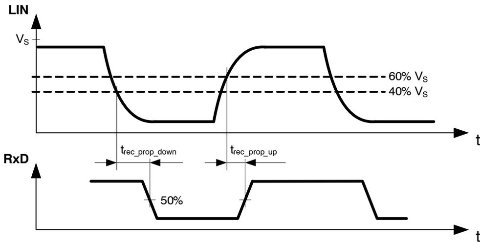
Figure 14. Definition of LIN Receiver Timing Parameters
