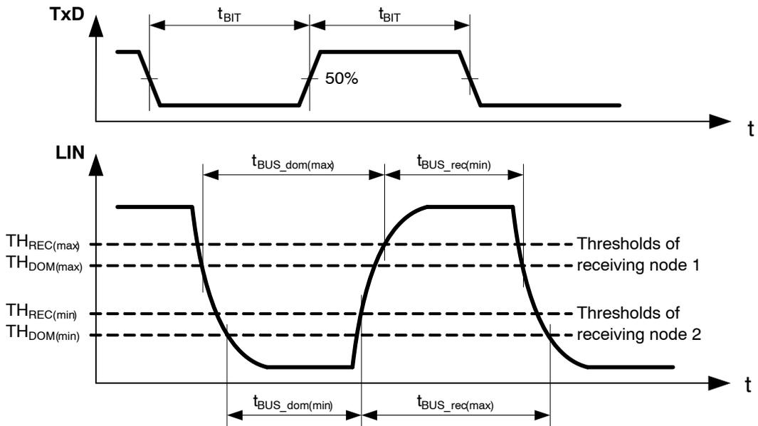
Figure 11. Definition of LIN Duty Cycle Parameters
