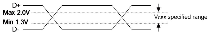
\*5: They indicate rise time ( $T_{RISE}$ ) and fall time ( $T_{FALL}$ ) of the full-speed differential data signal. They are defined by the time between 10% and 90% of the output signal voltage. For full-speed buffer,  $t_R/t_F$  ratio is regulated as within  $\pm 10\%$  to minimize RFI emission.
