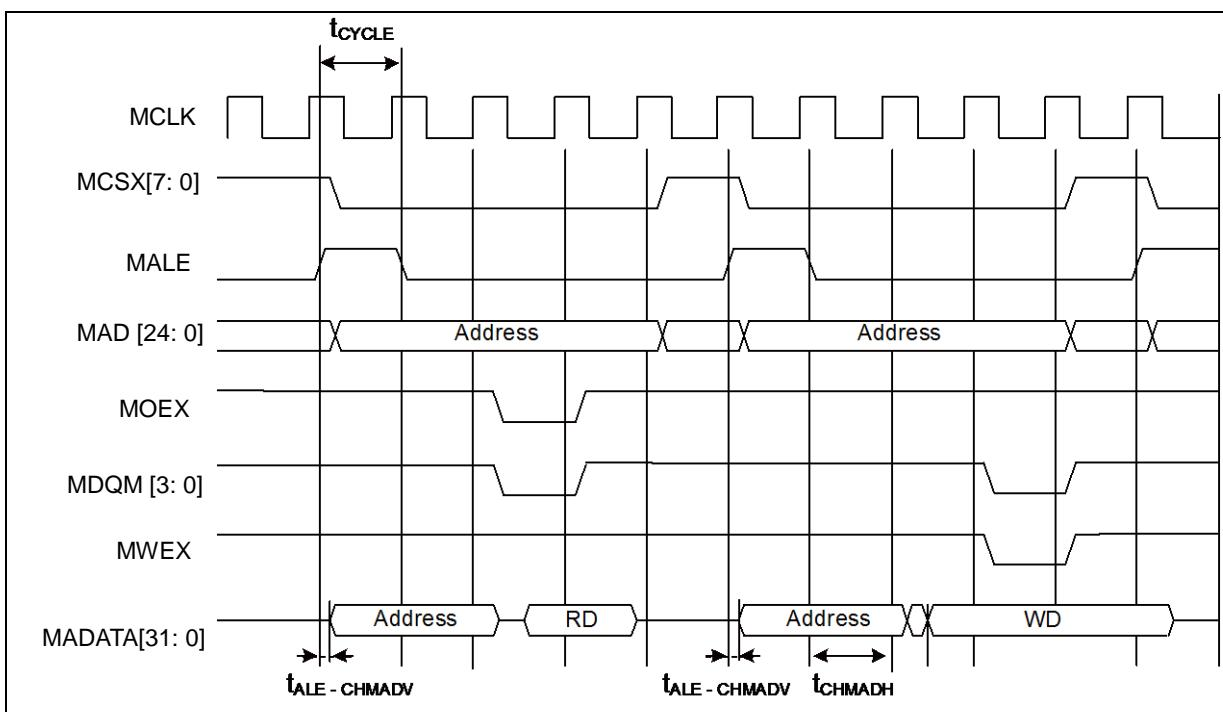
**Multiplexed Bus Access Synchronous SRAM Mode**
