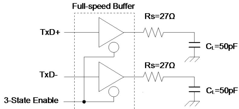
\*6: USB Full-speed connection is performed via twisted-pair cable shield with  $90\ \Omega \pm 15\%$  characteristic impedance (differential mode).
