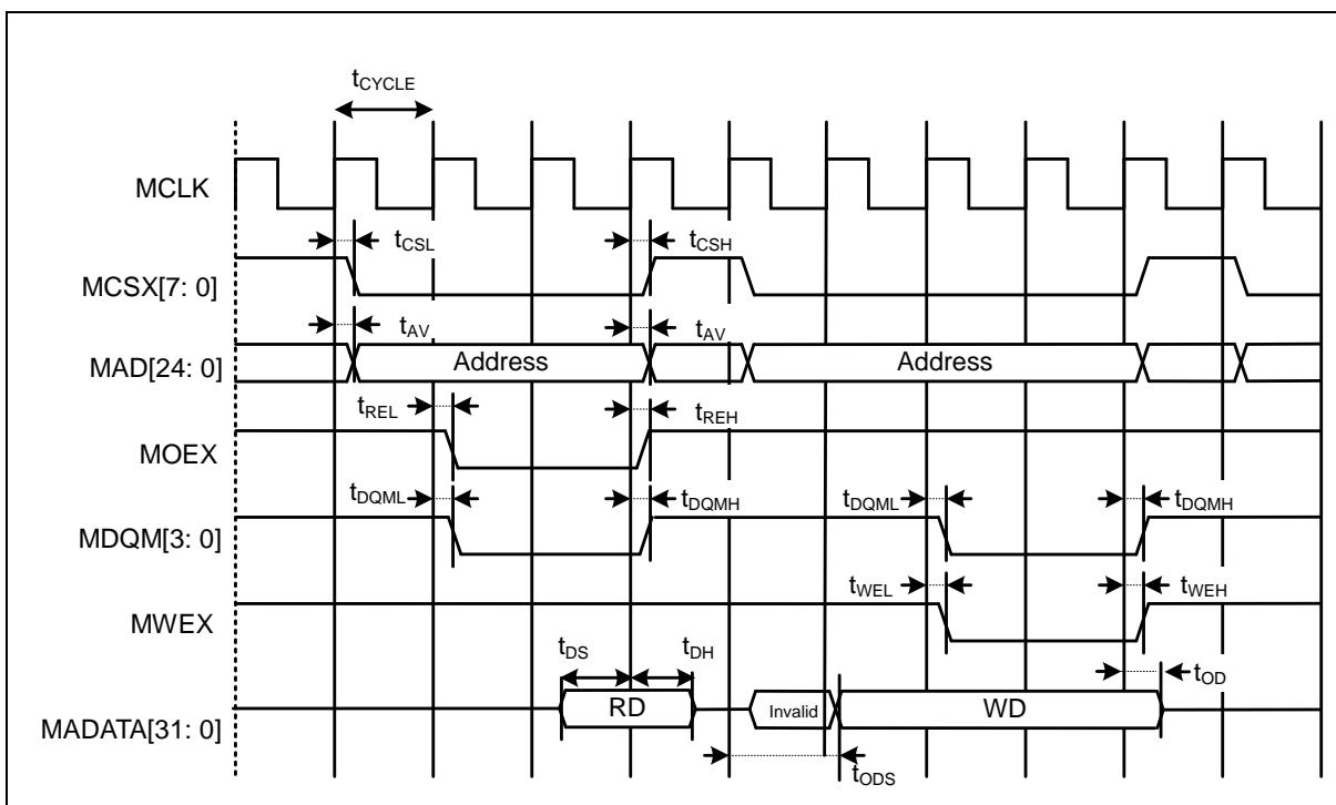
**Multiplexed Bus Access Asynchronous SRAM Mode**
