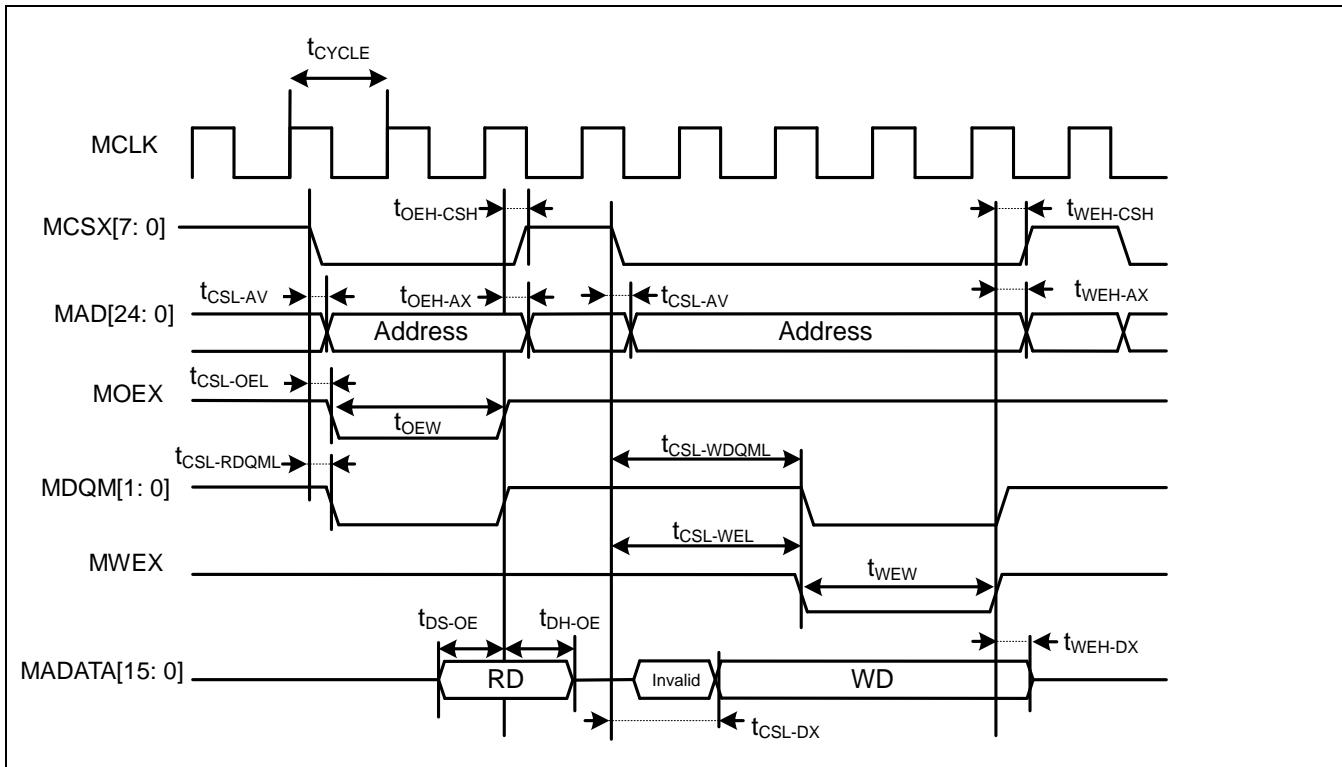
**Separate Bus Access Synchronous SRAM Mode**
