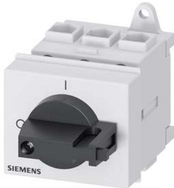
SENTRON, Switch disconnecter 3LD, main switch, 3-pole, Iu: 32 A, Operating power / at AC-23 A at 400 V: 11.5 kW, installation in distribution boards, knob-operated mechanism, black, handle direct at the switch
