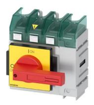
SENTRON, Molded case switch 3LD5 UL, Emergency switching-off, 4-pole, certified according to UL489 UL60947-4-1 and IEC60947-3, UL: 150A, SCCR 50kA at 480VAC, Operating power at 480VAC 3-phase: 100hp, IEC: 160A, Operating power at AC-23A at 400V: 75kW, floor mounting with direct handle, red/yellow, incl. terminal covers for the infeed side
