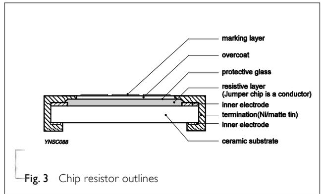
Fig. 3 Chip resistor outlines
