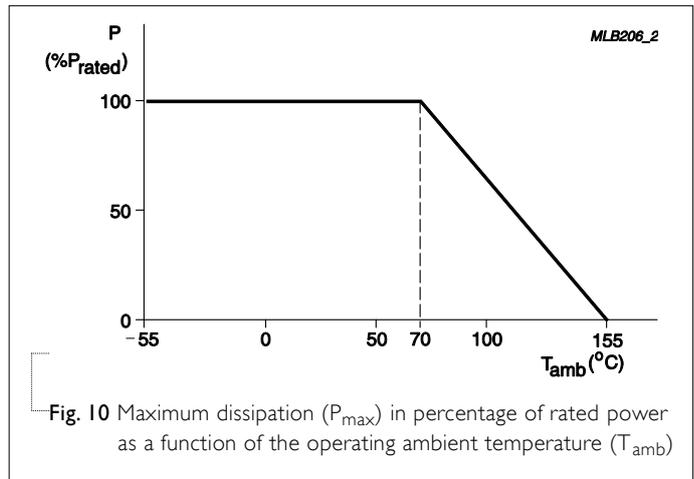
Fig. 10 Maximum dissipation (P<sub>max</sub>) in percentage of rated power as a function of the operating ambient temperature (T<sub>amb</sub>)
