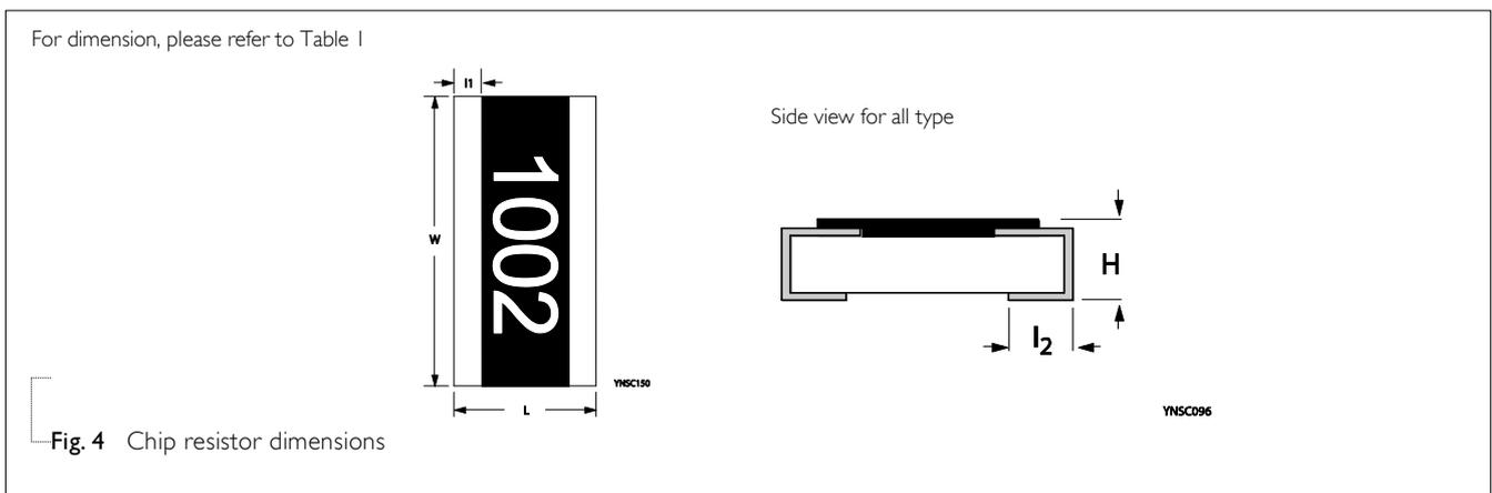
Fig. 4 Chip resistor dimensions
