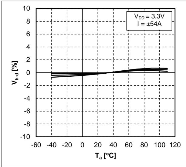
Figure 6. Temperature drift of sensitivity (for reference, n=3)
