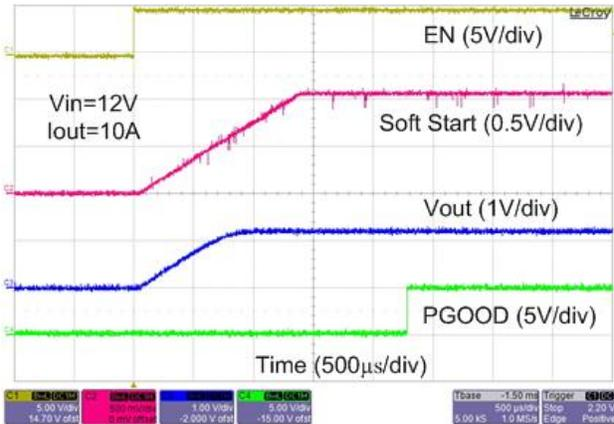
Figure 13. Startup Waveforms with 10 A Load Current
