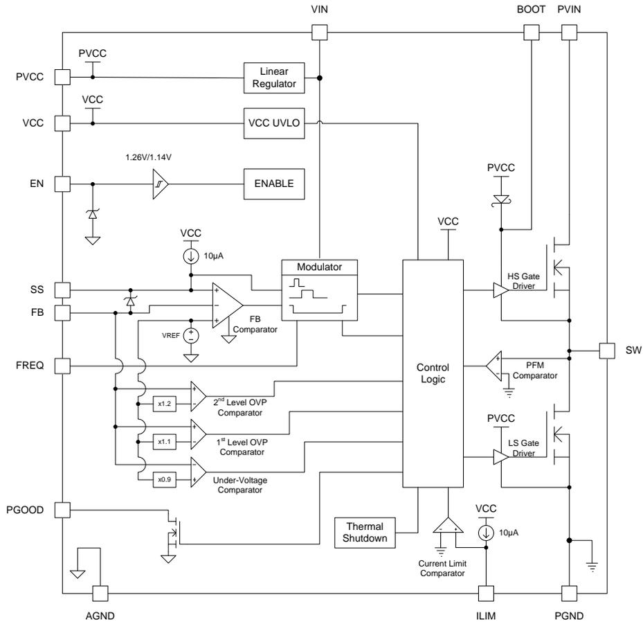
Figure 3. Block Diagram
