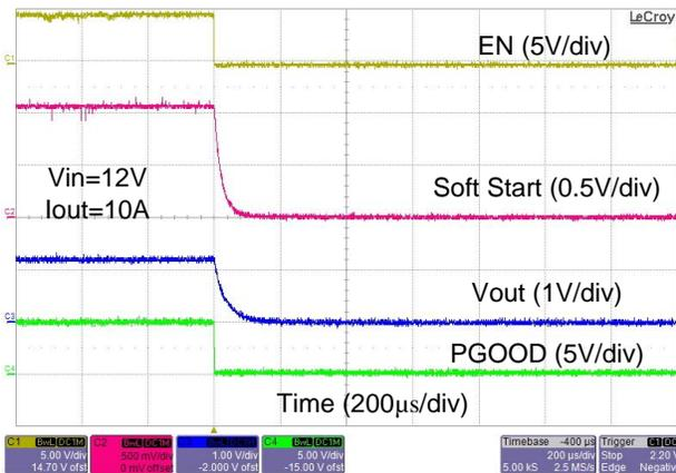
Figure 14. Shutdown Waveforms with 10 A Load Current
