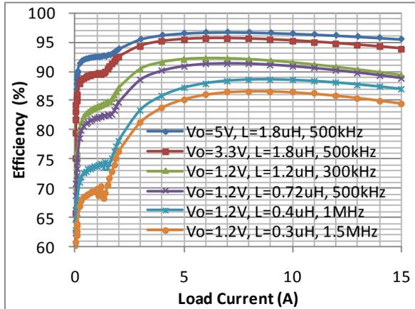
Figure 8. Efficiency vs. Load Current with  $V_{IN}=12\text{ V}$
