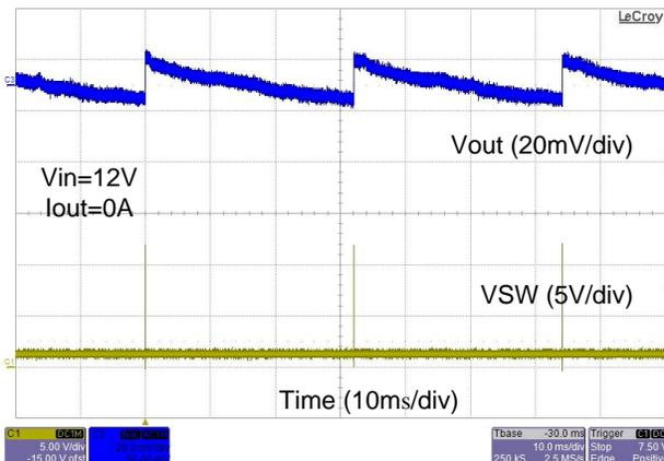
Figure 16. Static Load Ripple at Light Load
