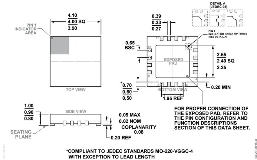
Figure 26. 16-Lead Lead Frame Chip Scale Package [LFCSP]
