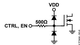
Figure 5. Digital Pins (CTRL and EN) Interface Schematic
