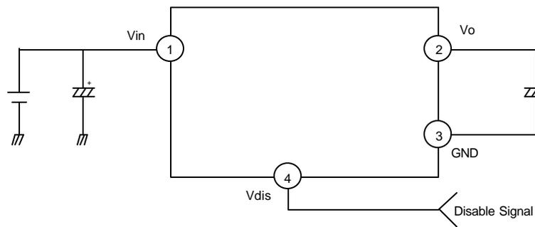
**Figure 1. Application Circuit**
