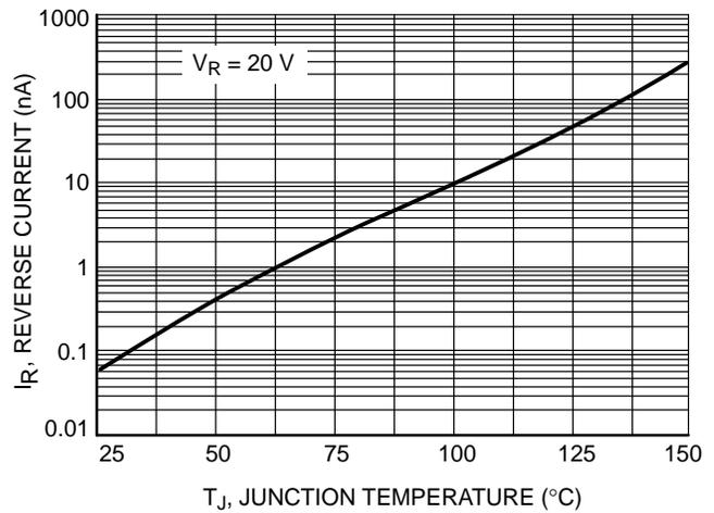
Figure 2. Typical Reverse Current versus Junction Temperature
