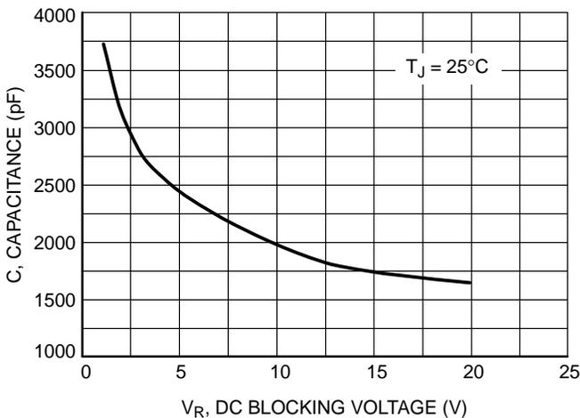
Figure 3. Typical Capacitance
