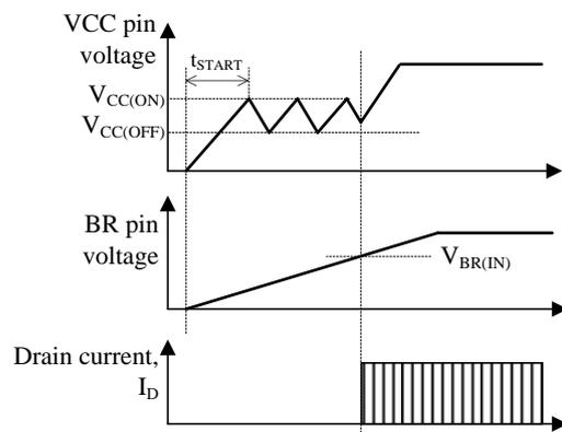
Figure 9-3 Startup operation (With Brown-In / Brown-Out Function)
