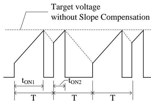
Figure 9-9 Drain current,  $I_D$ , waveform in subharmonic oscillation
