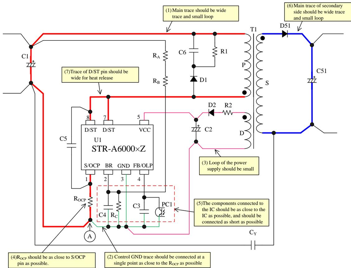
Figure 10-5 Peripheral circuit example around the IC
