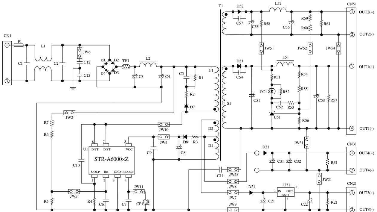
Figure 11-2 Circuit schematic for PCB circuit trace layout
