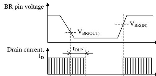
Figure 9-11 BR pin voltage and drain current waveforms
