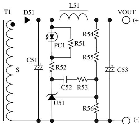
Figure 10-3 Peripheral circuit around secondary shunt regulator (U51)
