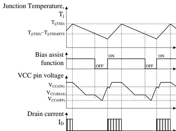
Figure 9-20 TSD operational waveforms
