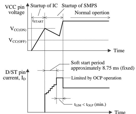
Figure 9-6 Vcc and  $I_D$  behavior during startup
