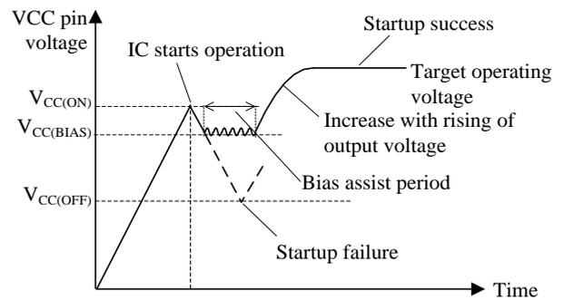
Figure 9-5 VCC pin voltage during startup period
