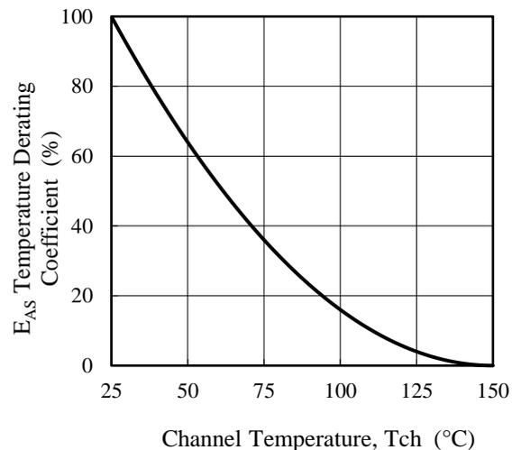
Figure 3-2 Avalanche Energy Derating Coefficient Curve
