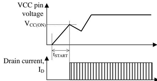
Figure 9-2 Startup operation (Without Brown-In / Brown-Out Function)
