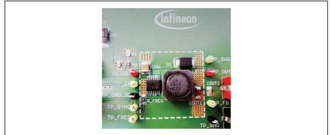
The buck-core is designed with the aim to be reproduced in customer applications (see dashed area in the right picture).
