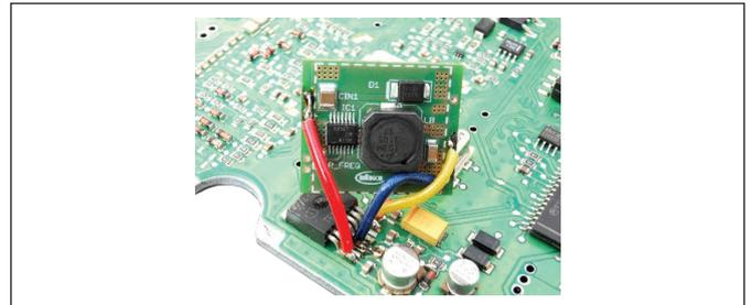
The buck-core is available as stand-alone 3-wire PCB. It can be easily applied in any application as replacement. Core characterization report and layout data (gerber-file) are available.
