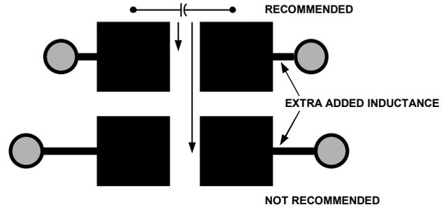
Figure 34. Recommended Pad Outline for Bypass Capacitors
