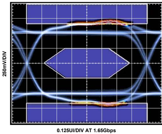
Figure 11. Tx Eye Diagram at TP2, PE = 6 dB
