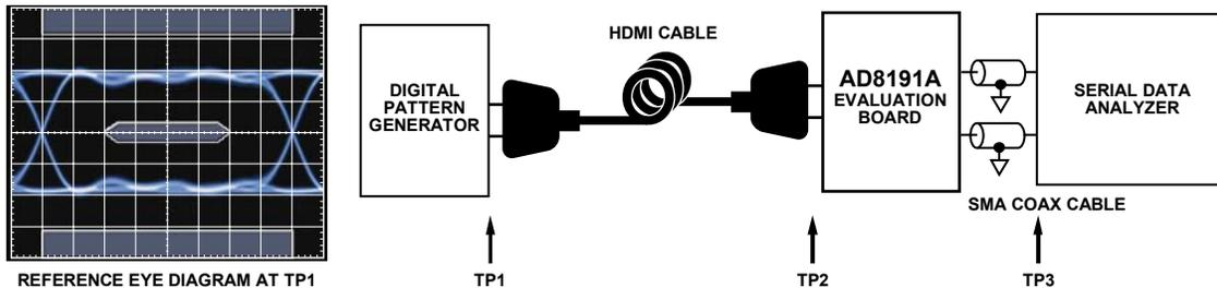
Figure 4. Test Circuit Diagram for Rx Eye Diagram
