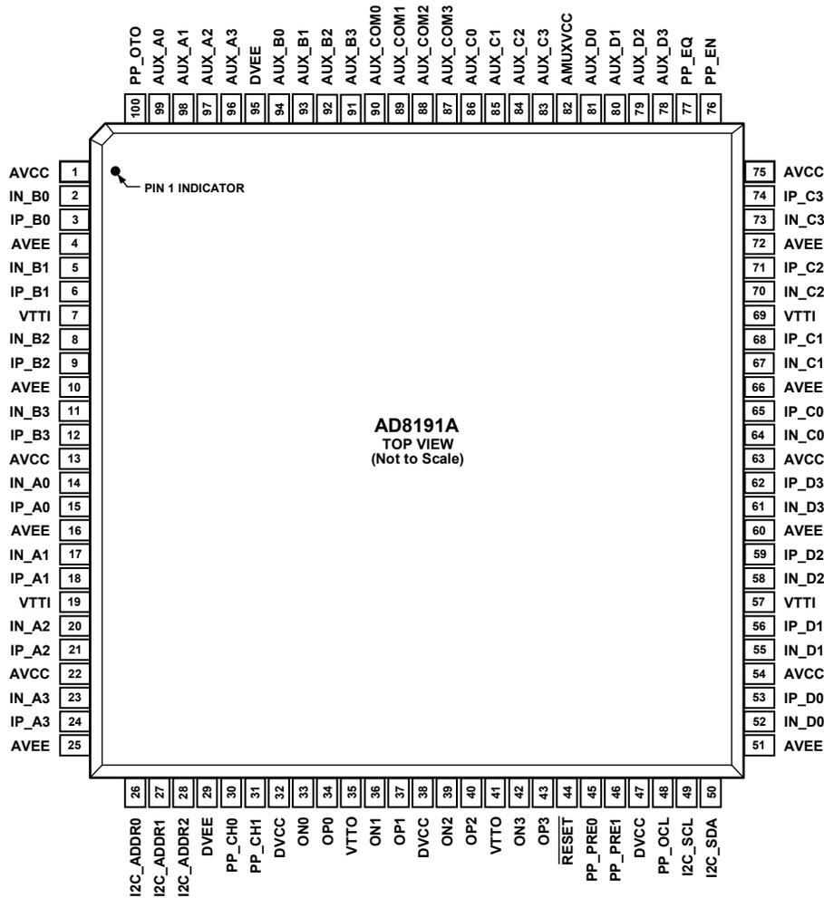
Figure 3. Pin Configuration
