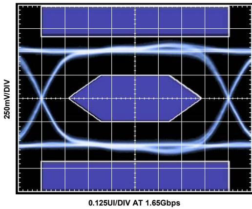
Figure 10. Tx Eye Diagram at TP2, PE = 2 dB
