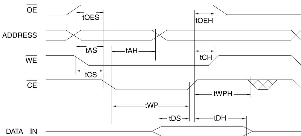
Note: 1. A complete sector (256 bytes) should be loaded using the waveforms shown in these byte load waveform diagrams.
