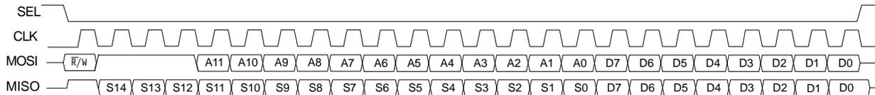
Figure 7. SPI 8 Bit Long Address Read/Write Access
