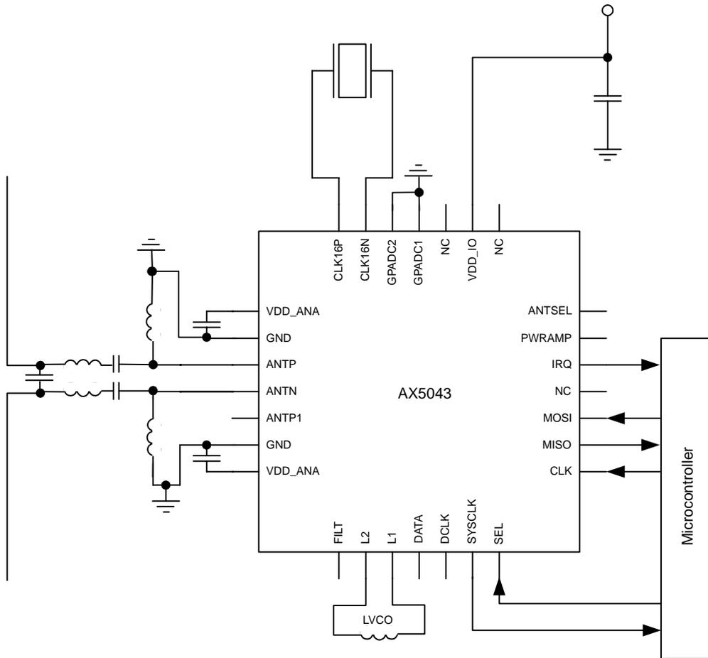
Figure 18. Typical Application Diagram with External VCO Inductor
