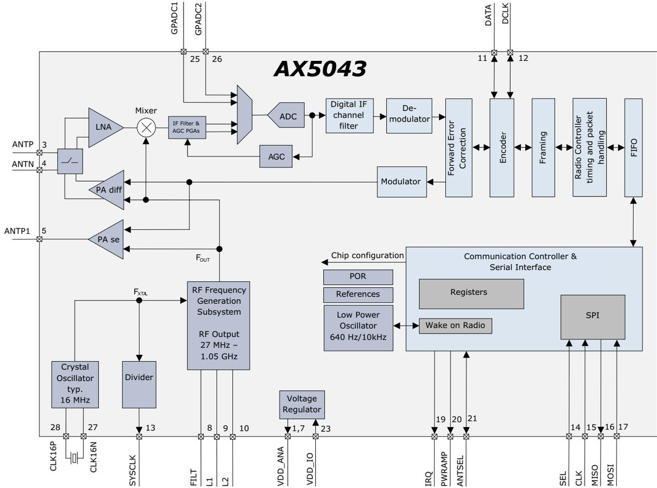
Figure 1. Functional Block Diagram of the AX5043
