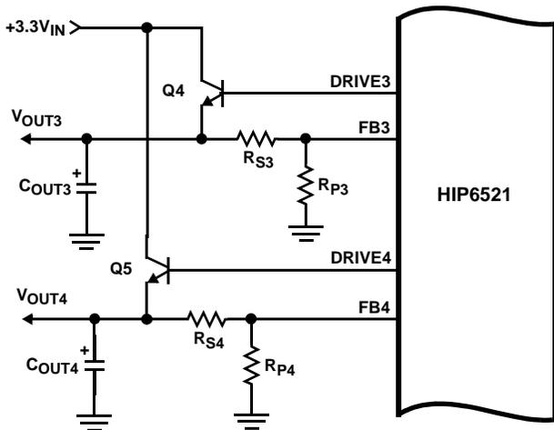
$$V_{OUT} = 0.8 \times \left( 1 + \frac{R_S}{R_P} \right)$$
