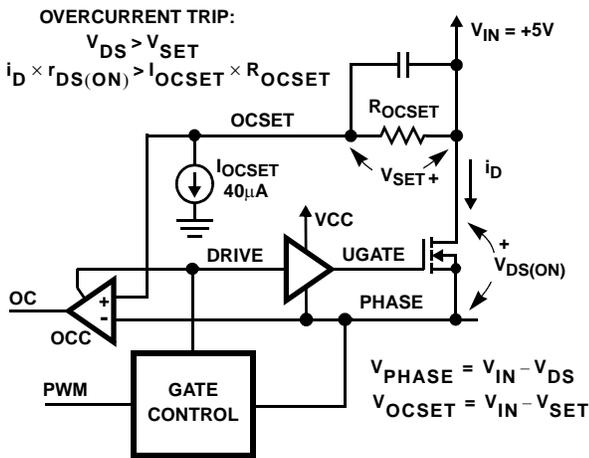
FIGURE 3. OVERCURRENT DETECTION
