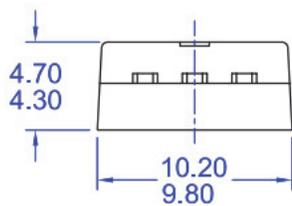
**Figure 16. TO220, Molded, 3-Lead, Jedec Variation AB**
