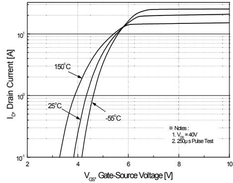
Figure 2. Transfer Characteristics
