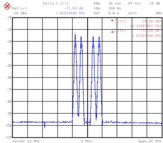
**FIGURE 6. FOUR GSM CARRIERS AT 12.4–15.6MHz,**
