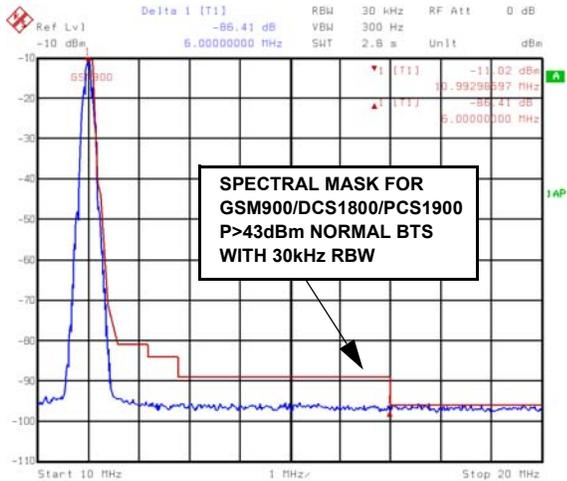
**FIGURE 3. GSM AT 11MHz, 78MSPS CLOCK**
