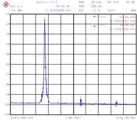
**FIGURE 4. GSM AT 11MHz, 78MSPS CLOCK**
