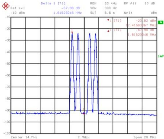
**FIGURE 5. FOUR EDGE CARRIERS AT 12.4–15.6MHz,**
