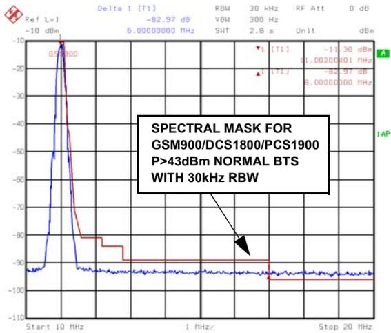
**FIGURE 1. EDGE AT 11MHz, 78MSPS CLOCK**
