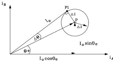
Fig. 3 Effect of Current Errors on Position
