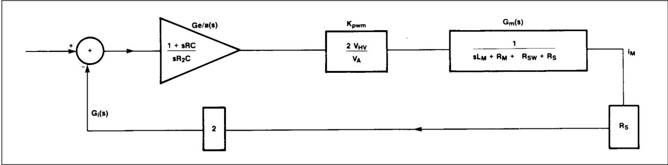
Fig. 11b Simplified laplace transform for stability analysis
