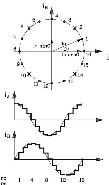
Fig. 2 Four Microstep per Step Drive Waveforms
