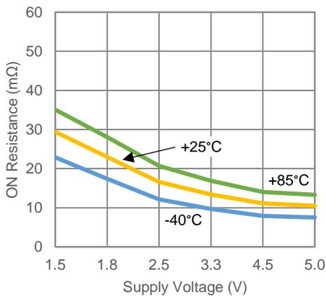
ON Resistance vs. Temperature (I<sub>OUT</sub> = 500mA)
