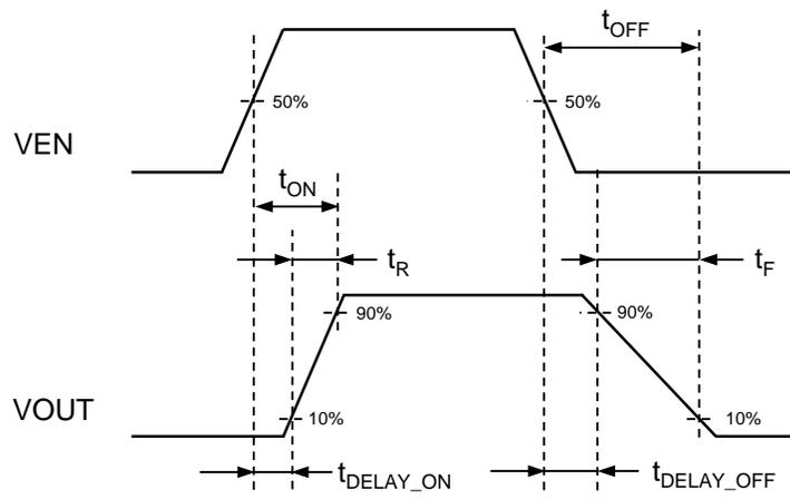
Figure 1. Timing Diagram
