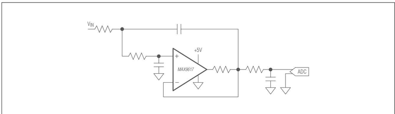
Figure 1. Typical Application Circuit: Sallen-Key Active Lowpass Filter
