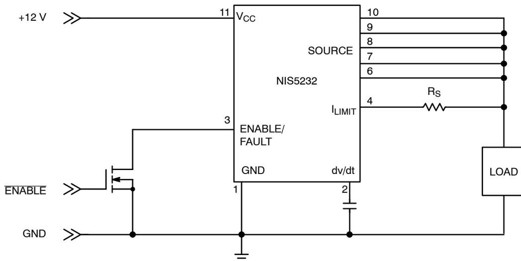
Figure 3. Application Circuit with Direct Current Sensing
