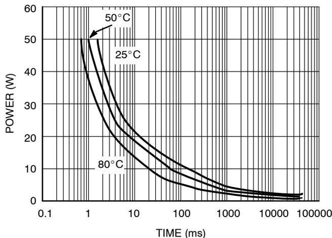
Figure 2. Power Dissipation vs. Thermal Trip Time
