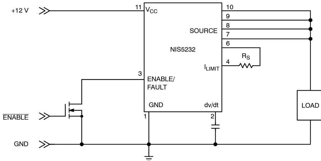
Figure 4. Application Circuit with Kelvin Current Sensing
