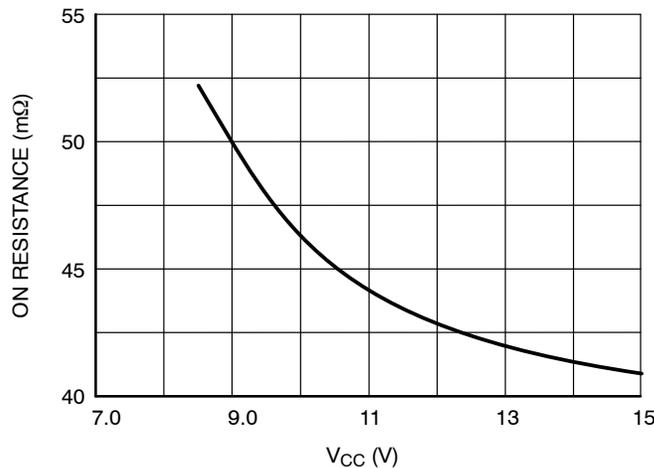
Figure 18. On Resistance vs. V<sub>CC</sub>
