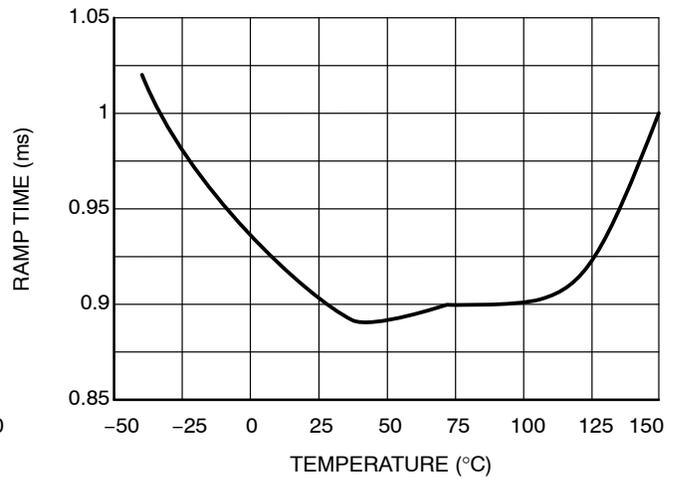
Figure 9. Output Voltage dv/dt Rate
