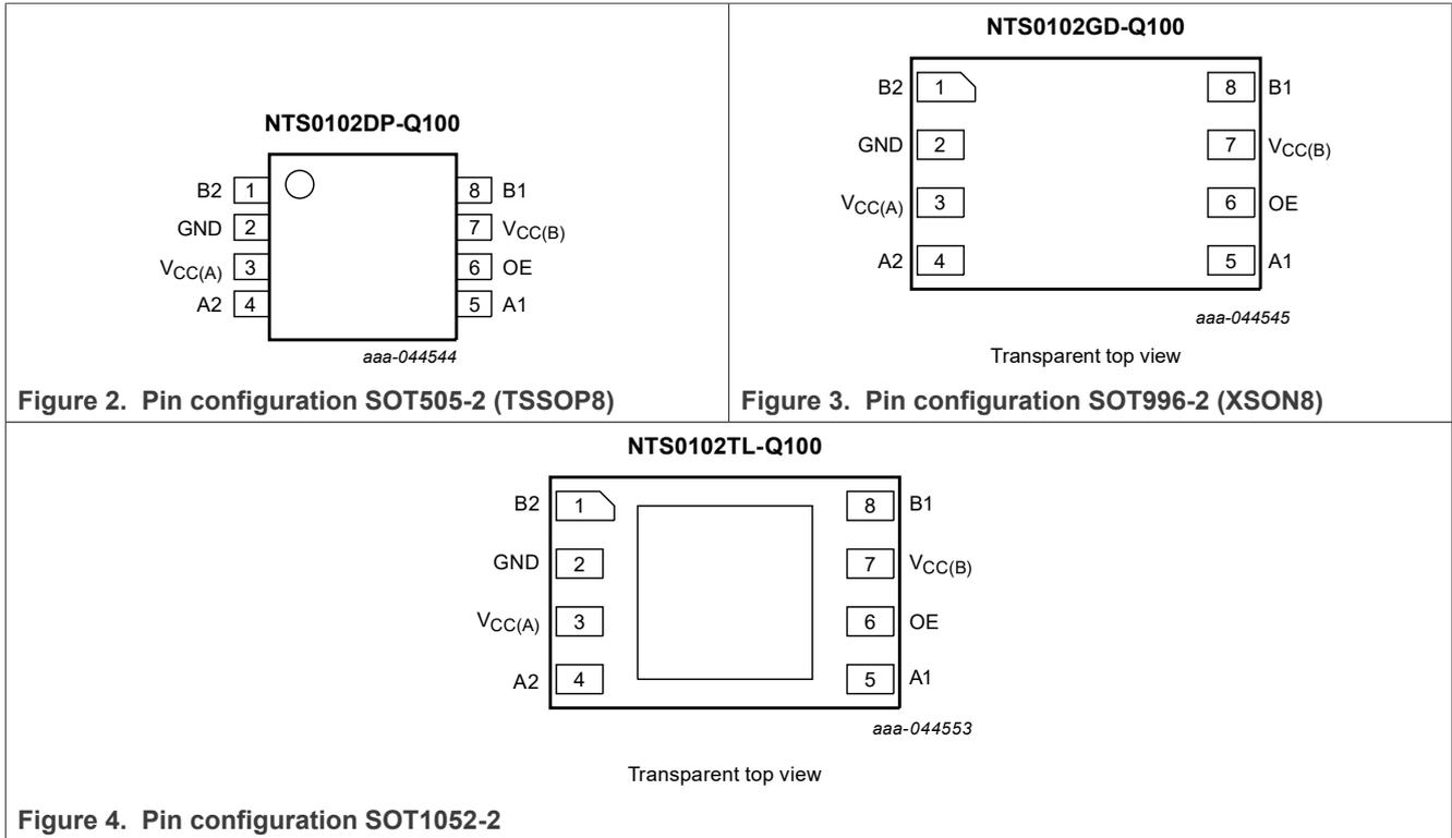
Figure 2. Pin configuration SOT505-2 (TSSOP8)
