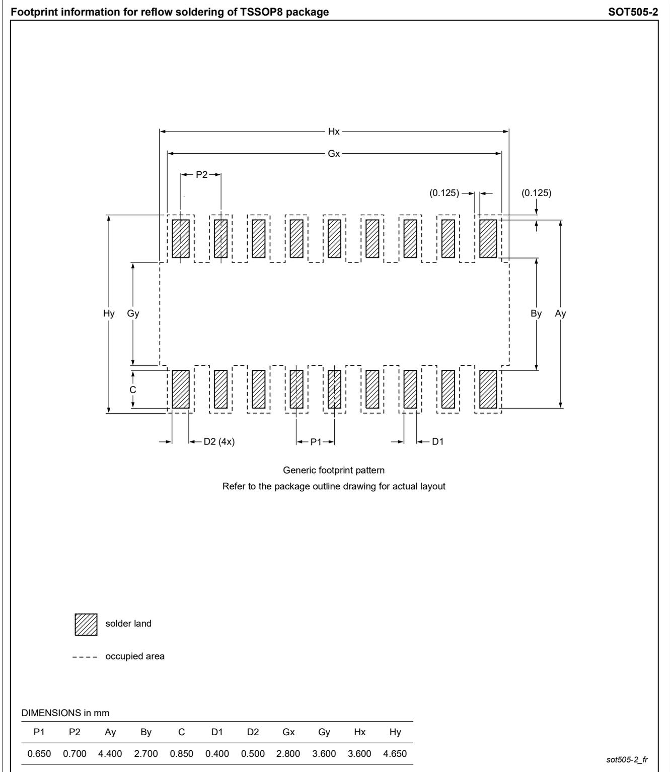
Figure 15. PCB footprint for SOT505-2 (TSSOP8); reflow soldering
