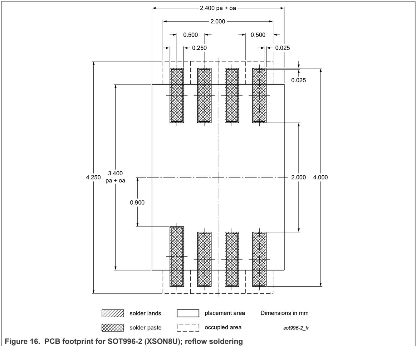
Figure 16. PCB footprint for SOT996-2 (XSON8U); reflow soldering
