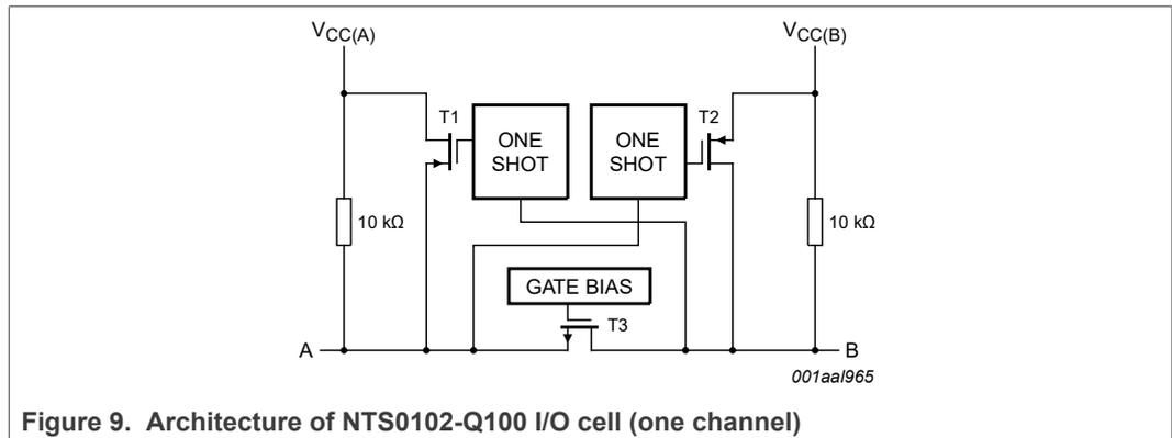
Figure 9. Architecture of NTS0102-Q100 I/O cell (one channel)
