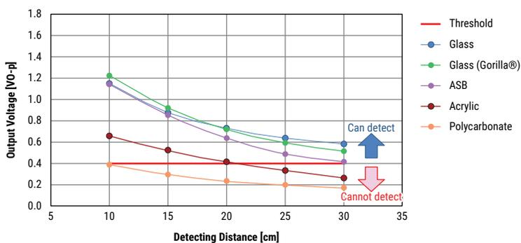
Measuring conditions: Transfer velocity - 1 m/s
