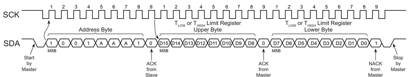
Note: Assumes the Pointer Register was previously set to point to the  $T_{LOW}$  or  $T_{HIGH}$  Limit Register.
