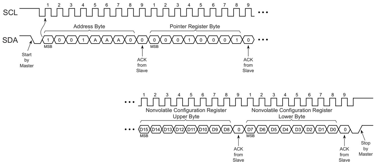
**Figure 6-7. Read from Nonvolatile Configuration Register**
