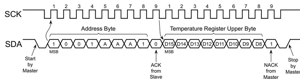
Note: Assumes the Pointer Register was previously set to point to the Temperature Register.
