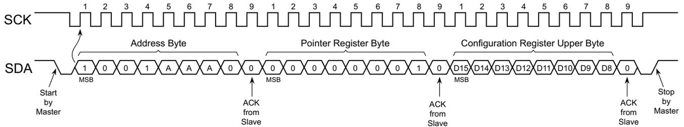
**Figure 6-5. Read from Configuration Register**
