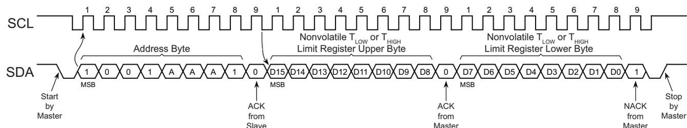
Note: Assumes the Pointer Register was previously set to point to the Nonvolatile T<sub>LOW</sub> or T<sub>HIGH</sub> Limit Register.
