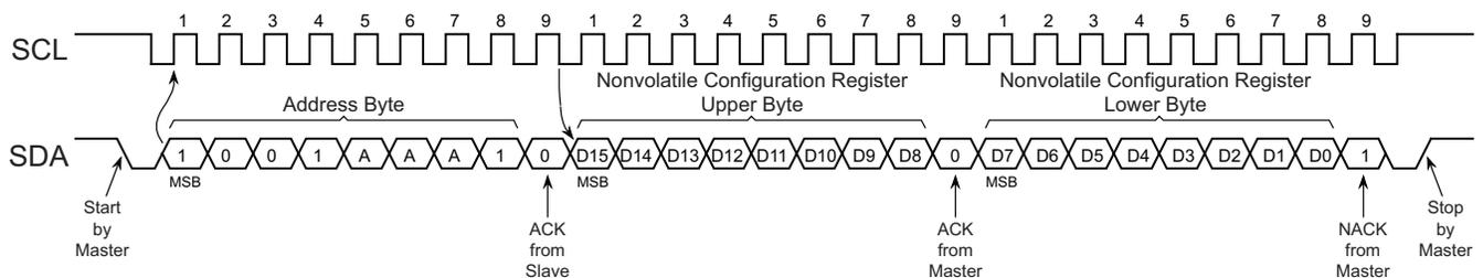
Note: Assumes the Pointer Register was previously set to point to the Nonvolatile Configuration Register.
