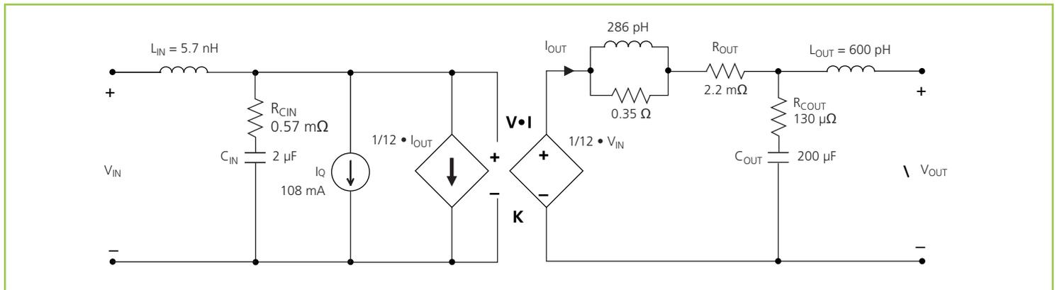
Figure 13 — V•I Chip™ module AC model
