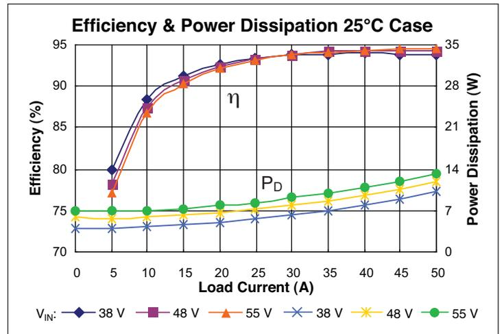
Figure 5 — Efficiency and power dissipation at  $T_C = 25^\circ\text{C}$
