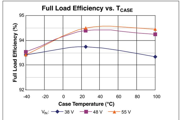
Figure 3 — Full load efficiency vs. temperature;  $V_{IN}$
