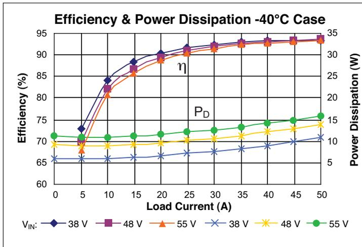
Figure 4 — Efficiency and power dissipation at  $T_C = -40^\circ\text{C}$
