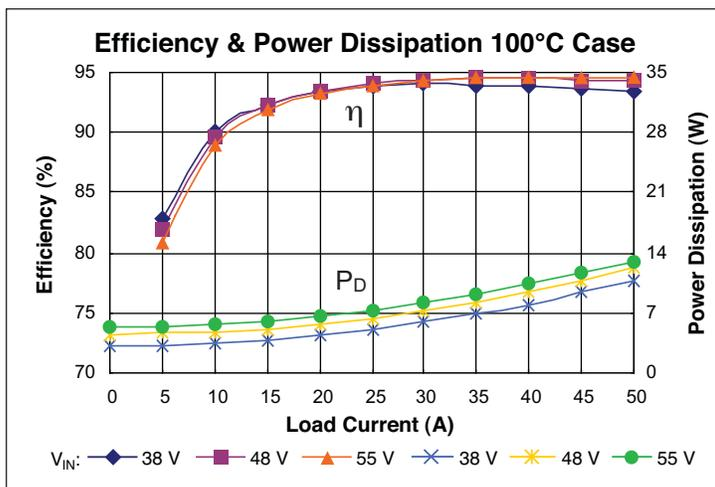
Figure 6 — Efficiency and power dissipation at  $T_C = 100^\circ\text{C}$
