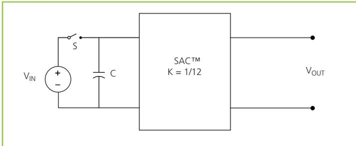
**Figure 15** — Sine Amplitude Converter™ with input capacitor
