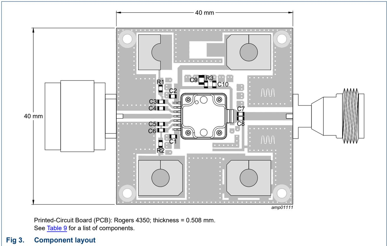
**Table 9. Demo test circuit list of components**
