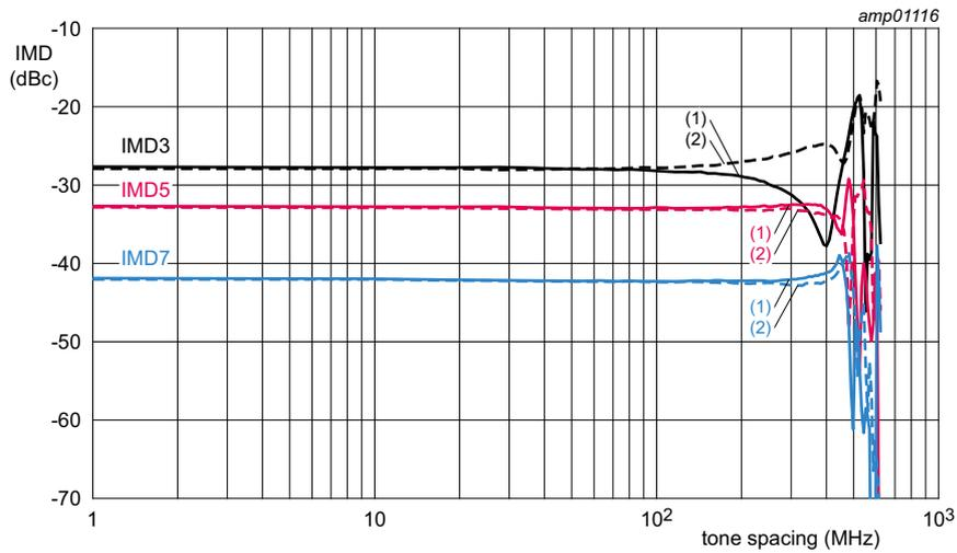
$T_{case} = 25\text{ }^{\circ}\text{C}$ ;  $V_{DS} = 30\text{ V}$ ;  $I_{Dq1} + I_{Dq2} = 91\text{ mA}$  (carrier and peaking stages);
