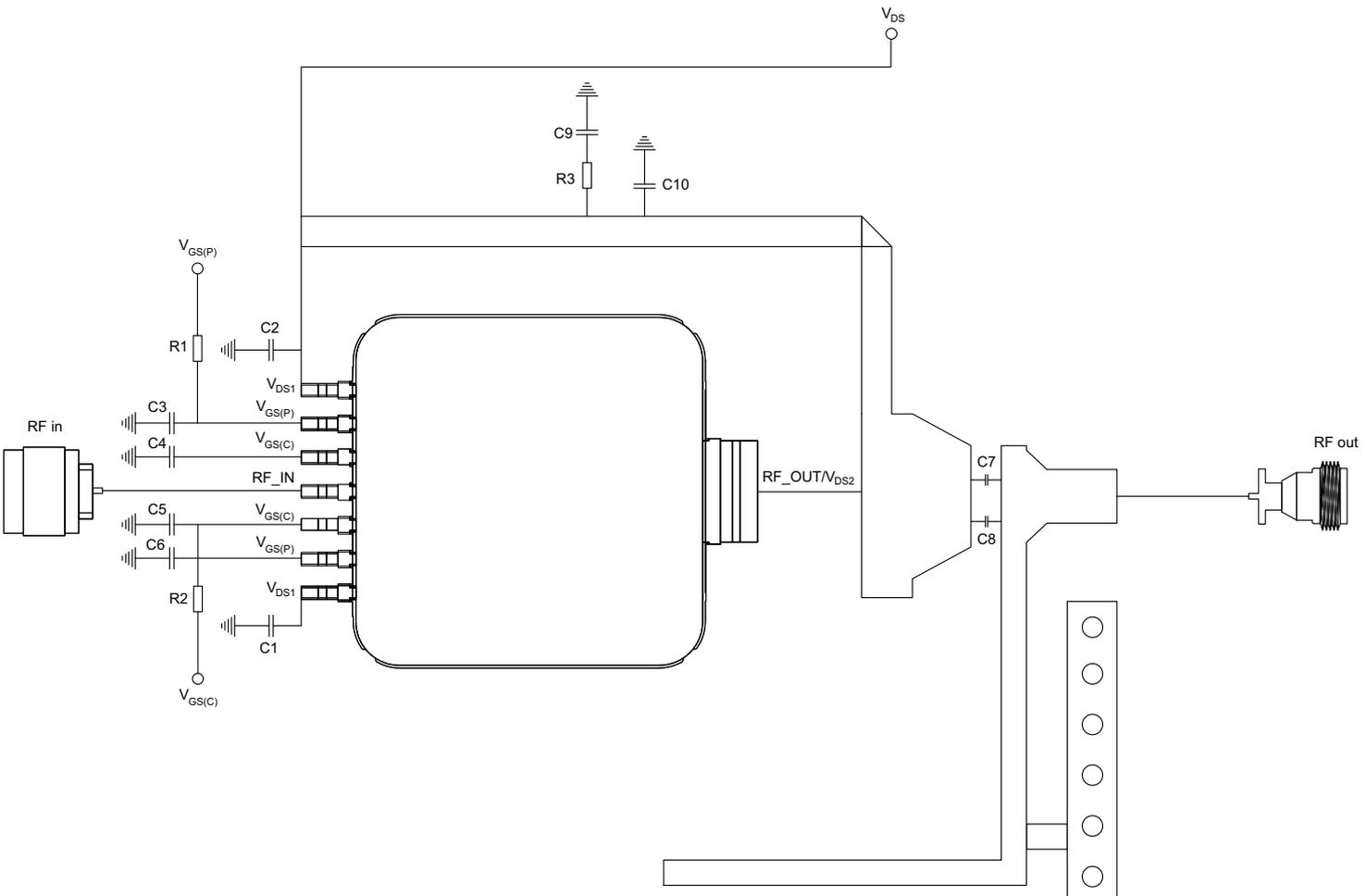
Fig 4. Electrical schematic
