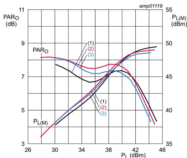
$T_{case} = 25\text{ }^{\circ}\text{C}$ ;  $V_{DS} = 30\text{ V}$ ;  $I_{Dq1} + I_{Dq2} = 91\text{ mA}$  (carrier and peaking stages);
