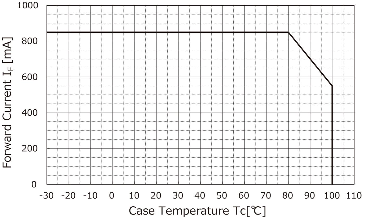
(Note) To keep the case temperature lower than the rating, enough heat-radiation performance needs to be secured by using an adequate heat sink (refer to section 7-③).
