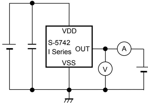
**Figure 7 Test Circuit 3**
