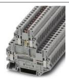
Component terminal block, Cross section: 0.14 mm² - 4 mm², AWG: 26 - 12, Connection type: Screw connection, Width: 5.2 mm, Color: gray, Mounting type: NS 35/7,5, NS 35/15
