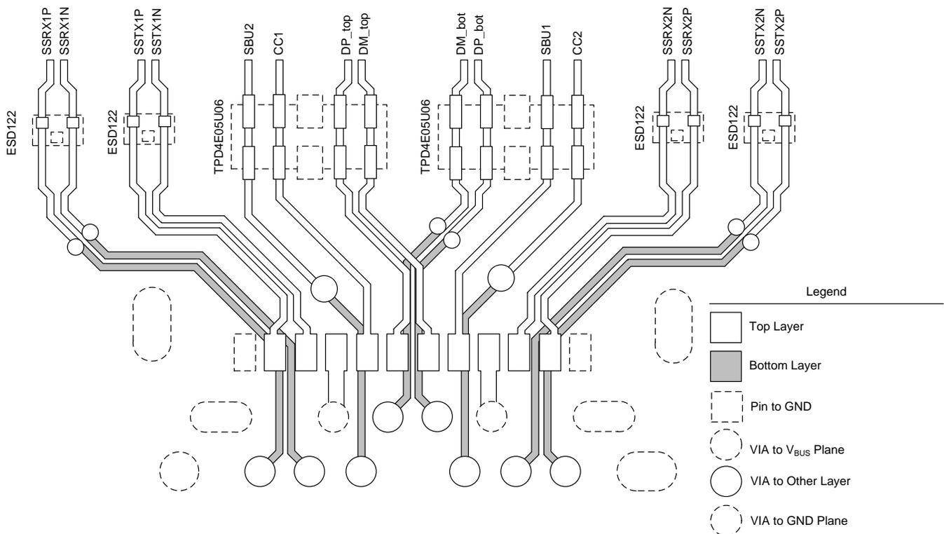
Figure 19. USB 3.1 Gen 2 SuperSpeed Lines Protected by ESD122
