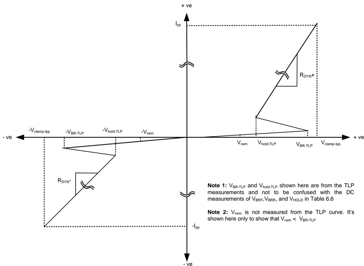
Figure 12. Generic TLP I-V Curve for a Bi-Directional ESD Device
