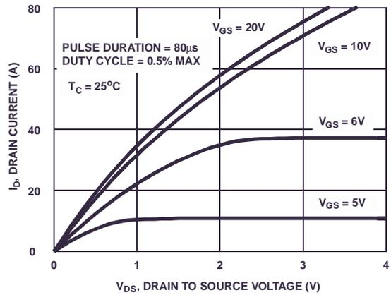
**Figure 8. Saturation Characteristics**
