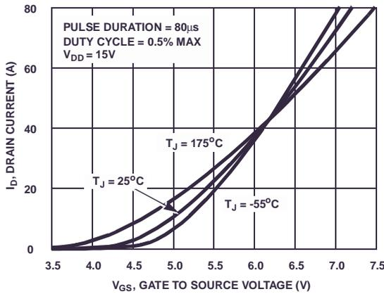
**Figure 7. Transfer Characteristics**
