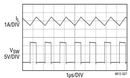
$12V_{IN}$  TO  $5V_{OUT}$  AT 2A
