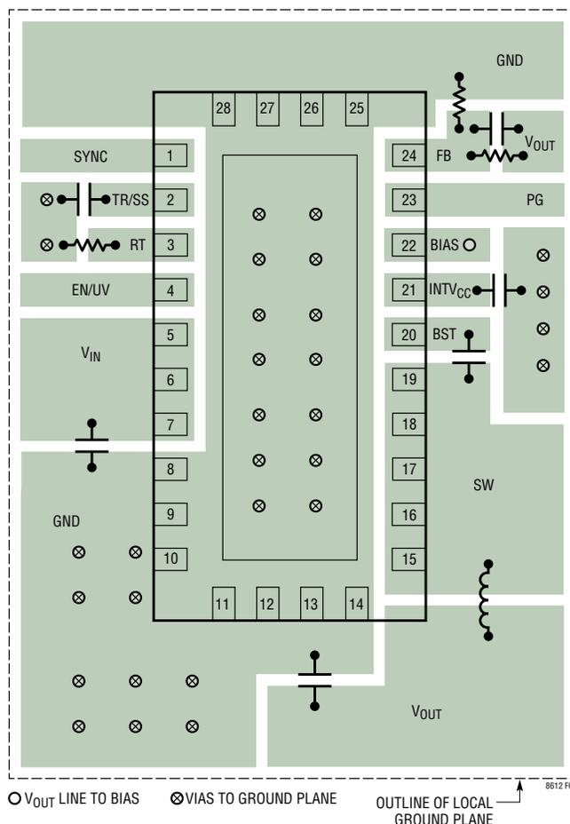
Figure 4. Recommended PCB Layout for the LT8612
