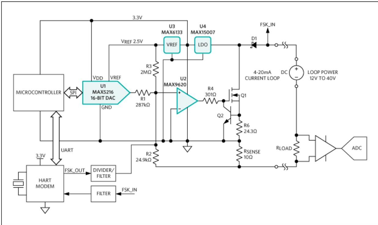
Figure 12. Block diagram with HART modem.
