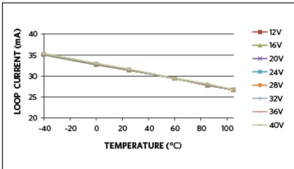
Figure 8. Current limit versus temperature with a 24.3Ω sense resistor.
