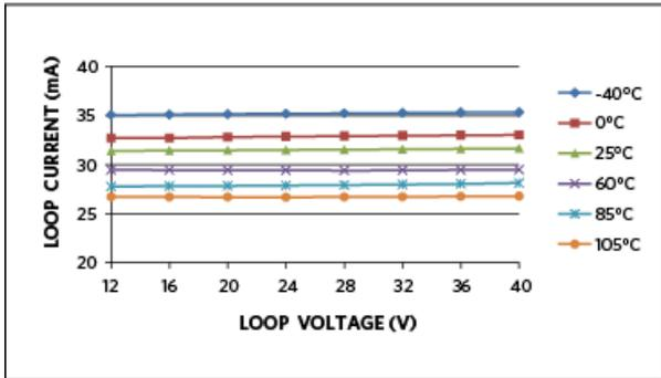
Figure 7. Current limit versus loop voltage with a 24.3Ω sense resistor.
