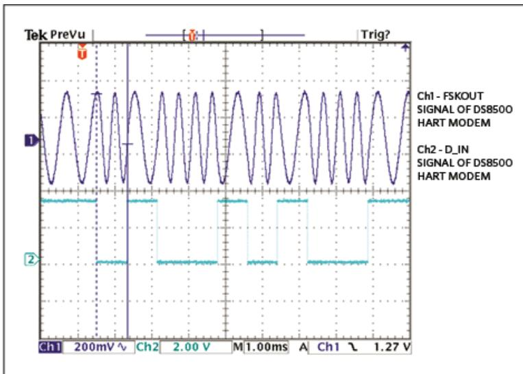
Figure 10. HART communication over a 4–20mA current loop.
