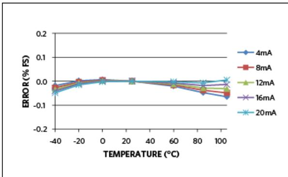
Figure 4. Transmitter error change versus temperature with a 12V loop supply.
