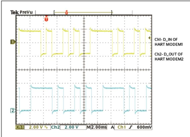
Figure 11. HART communication between two modems.
