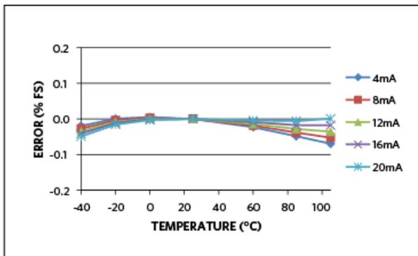
Figure 5. Transmitter error change versus temperature with a 24V loop supply.
