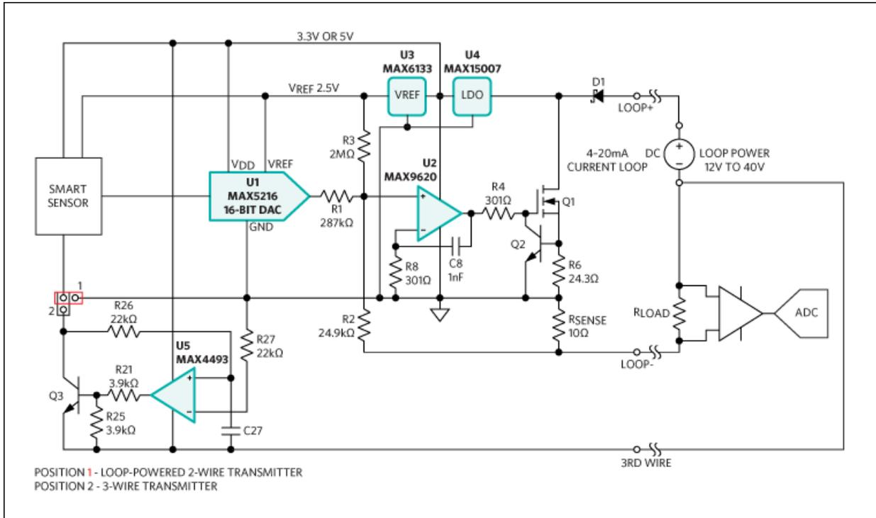
Figure 2. Block diagram for a universal 2- or 3-wire smart sensor transmitter.
