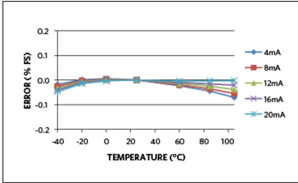
Figure 6. Transmitter error change versus temperature with a 36V loop supply.
