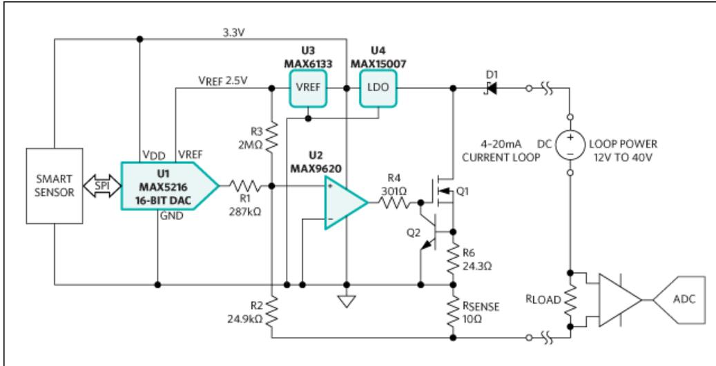
Figure 1. Reference design for a 4–20mA loop-powered transmitter features the MAX5216 16-bit DAC (U1), the MAX9620 op amp (U2), the MAX6133 voltage reference (U3), and the MAX15007 LDO (U4).
