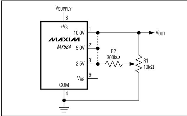
Figure 3. Fine Adjustment of Output Voltage ( $\pm 200\text{mV}$ )
