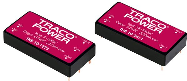
The THB 10 series is a range of high performance DC/DC converter modules with double reinforced insulation system. It complies to latest medical safety standard IEC 60950-1 3rd edition for MOOP (Means of Operator Protection). The product comes in a 2"x1" industry standard package. All 12 models features wide 2:1 input voltage range and fully regulated output voltage. The converters offer an economical solution for demanding applications in industrial and medical instrumentation.
