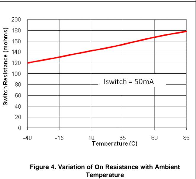
Figure 4. Variation of On Resistance with Ambient Temperature
