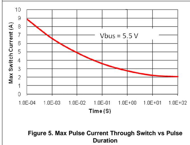
Figure 5. Max Pulse Current Through Switch vs Pulse Duration
