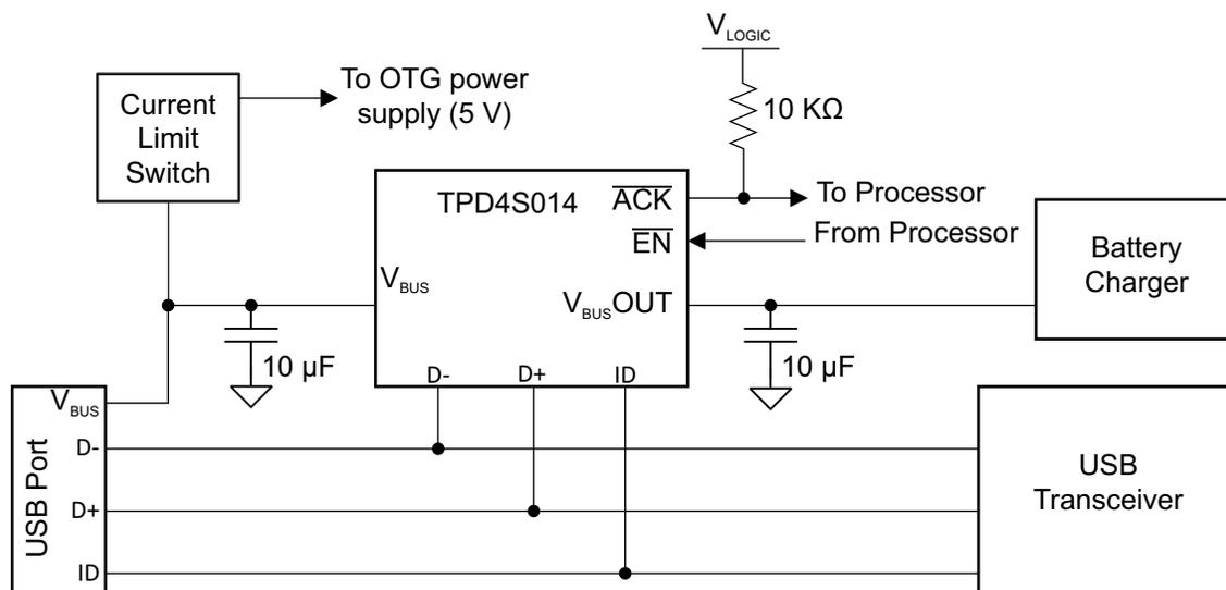
Figure 16. OTG Schematic
