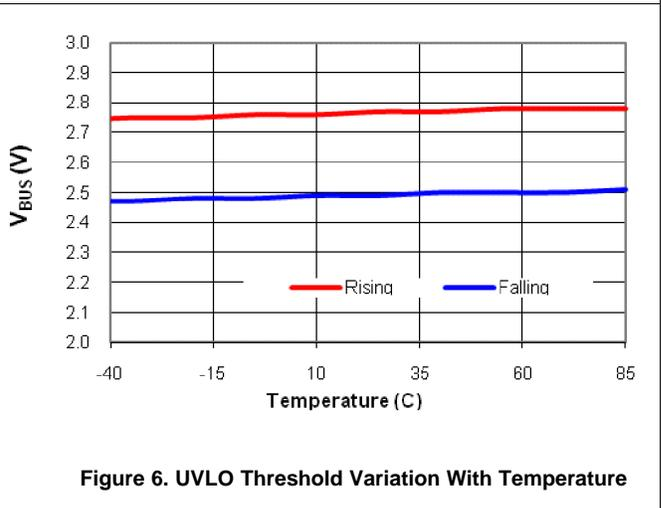
Figure 6. UVLO Threshold Variation With Temperature
