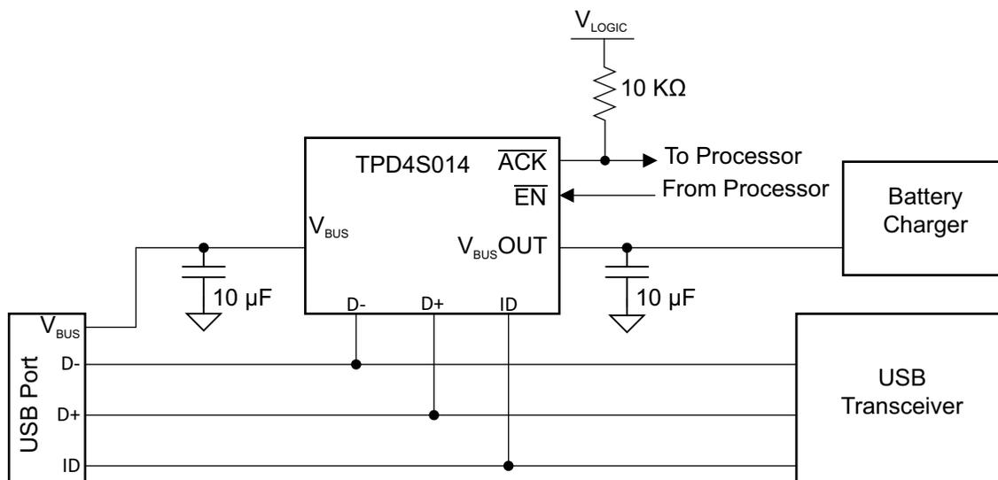
Figure 12. Non-OTG Schematic
