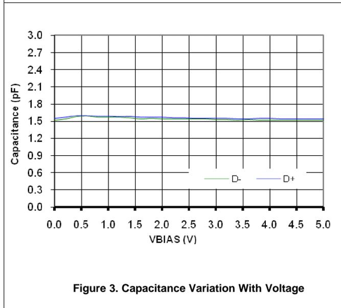
Figure 3. Capacitance Variation With Voltage
