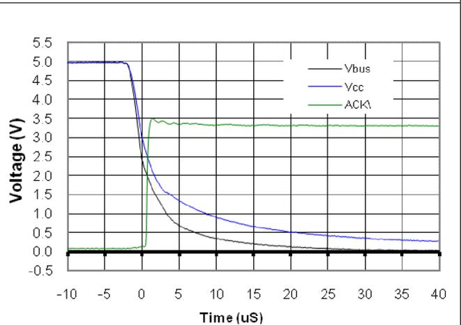
Figure 10. Device Turn OFF Characteristics (Undervoltage)
