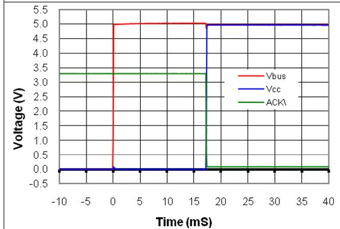
Figure 9. Device Turn on Characteristics
