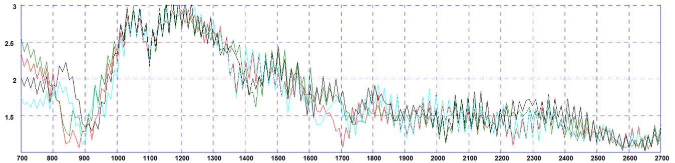
\*VSWR measured with no whip and 5m (16') of CS29 cable Black & Blue = no ground plane Green and Red = 600x 600mm (2'x2') ground plane
