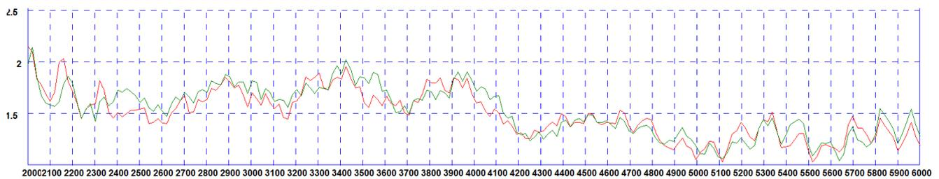
\*VSWR measured with no whip and 5m (16') of CS32 cable
