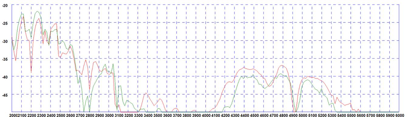
\*Isolation measured with no whip and 5m (16') of CS29 cable Red Plot = 600x600mm (2' X2') ground plane Green Plot = no ground plane
