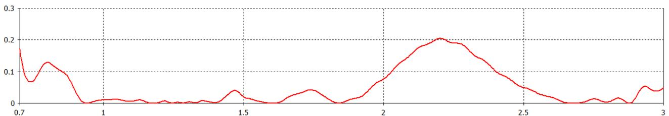
\*Correlation co-efficient simulated in free space with no whip, no additional cable and no ground plane
