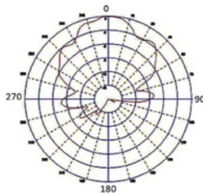
\*3D radiation patterns simulated in CST Microwave Studio on a 600x600mm (2' X2') ground plane with both elements fed together.
