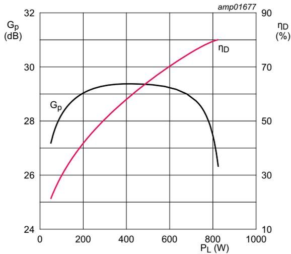
$V_{DS} = 55 \text{ V}$ ;  $I_{Dq} = 50 \text{ mA}$  per section;  $f = 108 \text{ MHz}$ .
