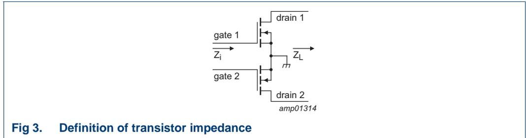
Fig 3. Definition of transistor impedance
