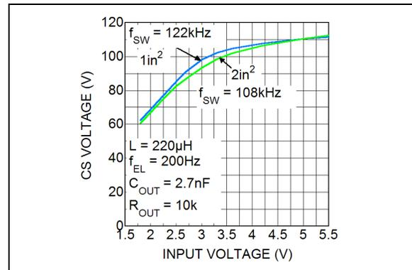
**FIGURE 2-6:** Peak CS Voltage vs. Input Voltage.
