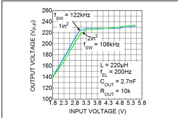
**FIGURE 2-7:** Peak Output Voltage vs. Input Voltage.
