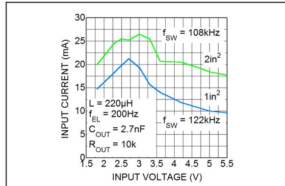
**FIGURE 2-5:** Total Input Current vs. Input Voltage.
