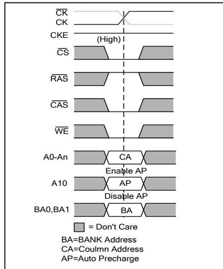
7.6.2 Basic Write Timing Parameters
