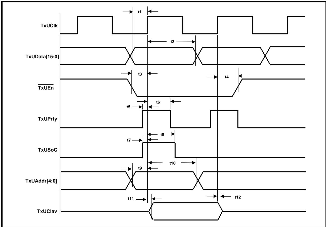
**FIGURE 5. GFC NIBBLE-FIELD SERIAL INPUT INTERFACE (AT TRANSMIT CELL PROCESSOR) TIMING**
