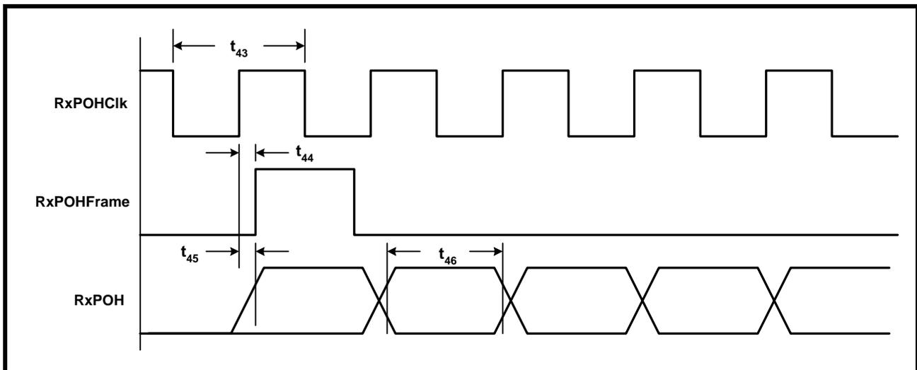
**FIGURE 14. GFC NIBBLE-FIELD SERIAL OUTPUT PORT TIMING (RECEIVE CELL PROCESSOR)**
