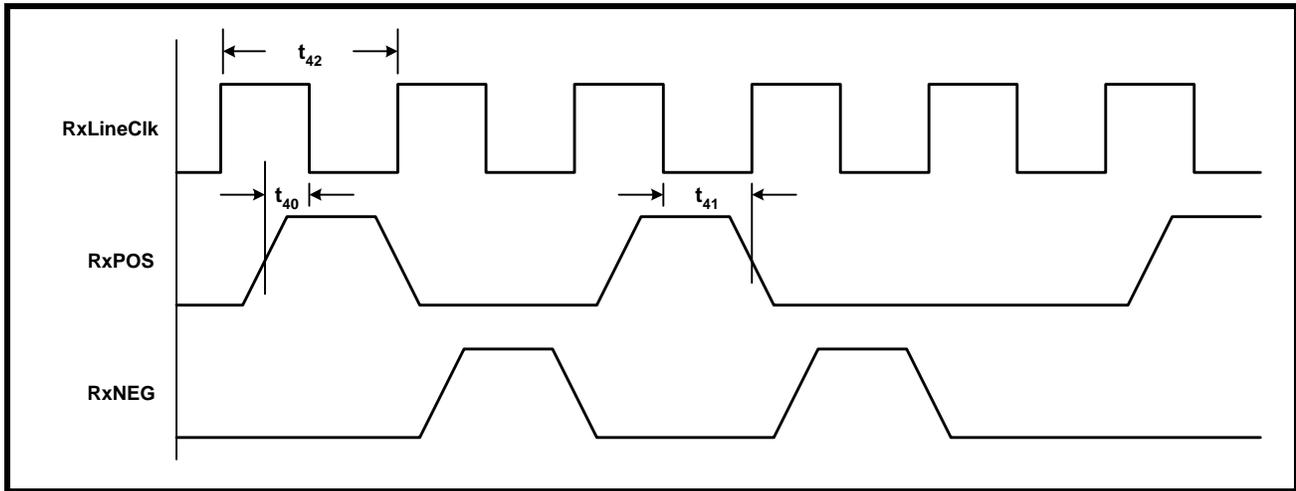
**FIGURE 13. RECEIVE PLCP PROCESSOR—POH BYTE SERIAL OUTPUT PORT INTERFACE TIMING**
