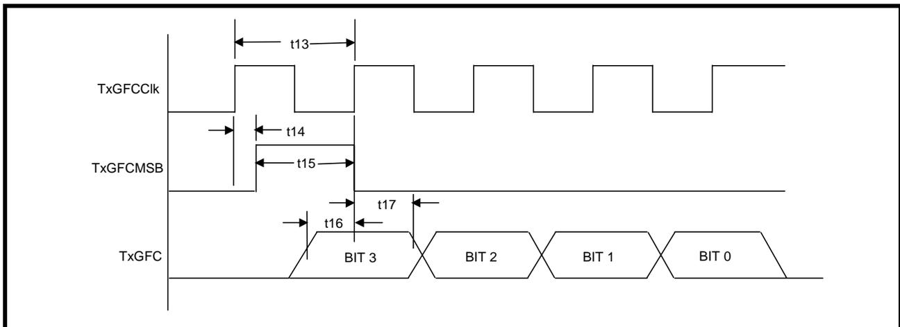
**FIGURE 6. TRANSMIT PLCP PROCESSOR—POH BYTE SERIAL INPUT PORT INTERFACE TIMING**
