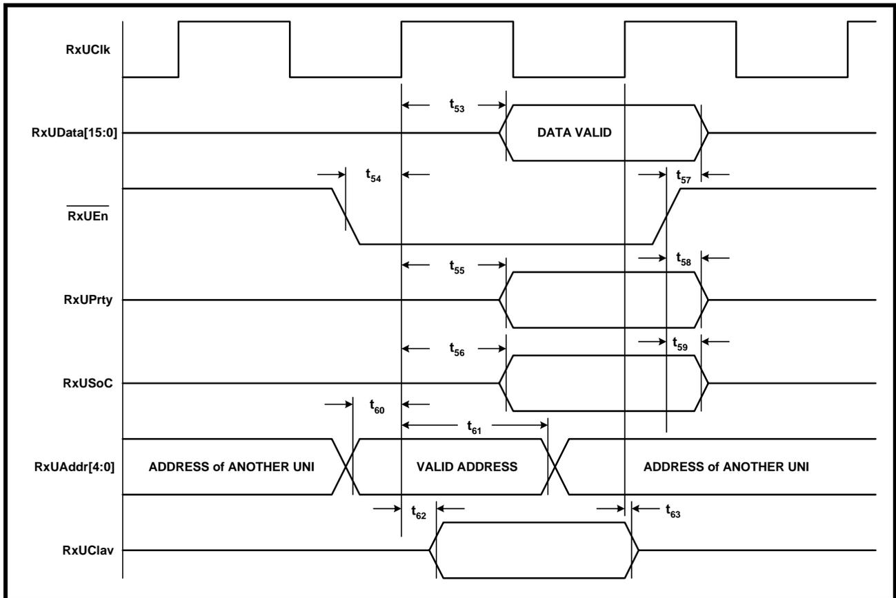
FIGURE 16. MICROPROCESSOR INTERFACE TIMING - INTEL TYPE PROGRAMMED I/O READ OPERATIONS
