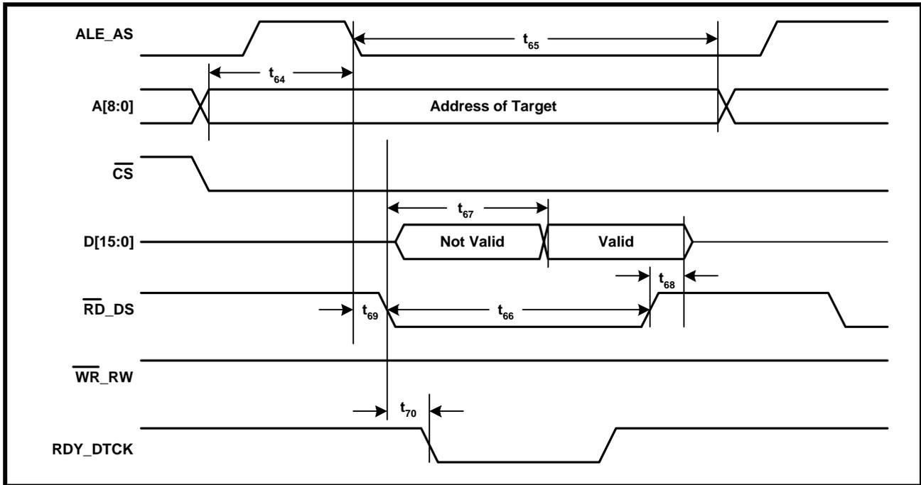
FIGURE 17. MICROPROCESSOR INTERFACE TIMING - INTEL TYPE PROGRAMMED I/O WRITE OPERATIONS
