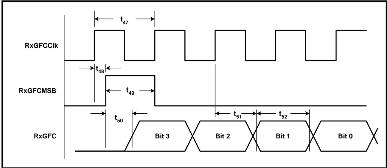
**FIGURE 15. RECEIVE UTOPIA INTERFACE BLOCK TIMING**
