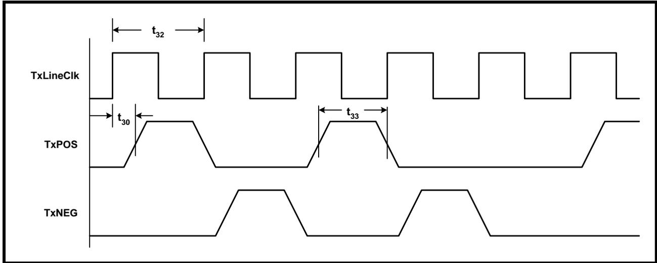
FIGURE 9. TRANSMIT DS3 FRAMER LINE INTERFACE OUTPUT TIMING (TxPOS AND TxNEG ARE UPDATED ON THE FALLING EDGE OF TxLINECLK)
