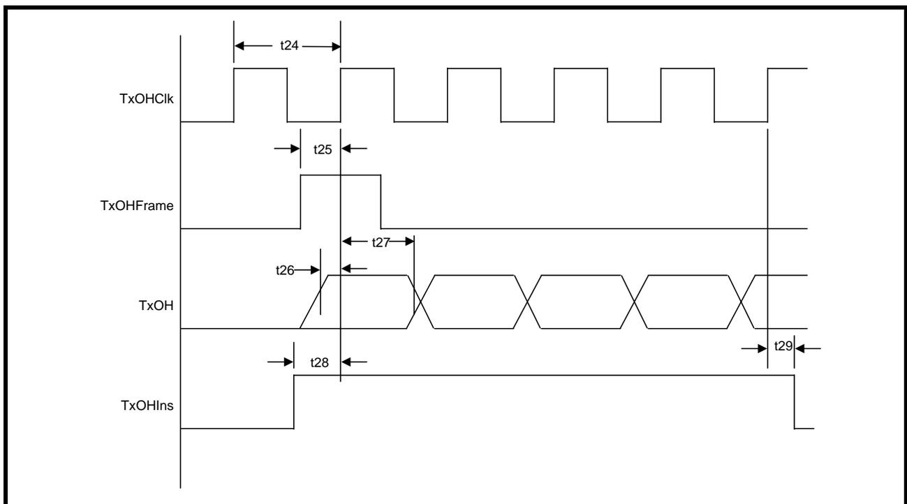
FIGURE 8. TRANSMIT DS3 FRAMER LINE INTERFACE OUTPUT TIMING (TxPOS AND TxNEG ARE UPDATED ON THE RISING EDGE OF TxLINECLK)
