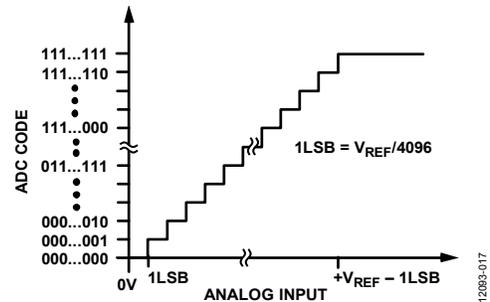
Figure 34. Transfer Characteristic
