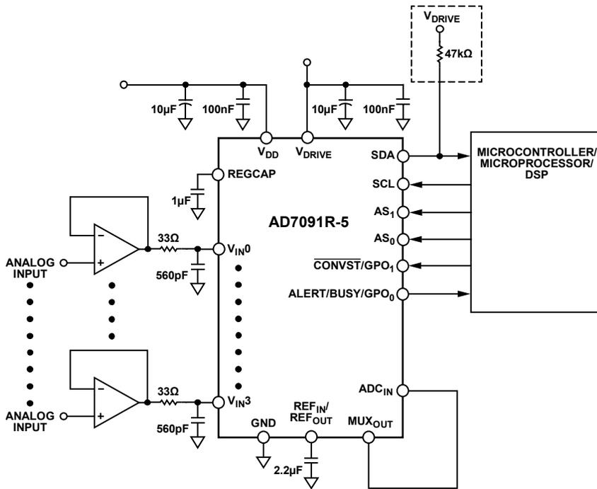
Figure 38. Typical Connection Diagram Without Optional Buffer
