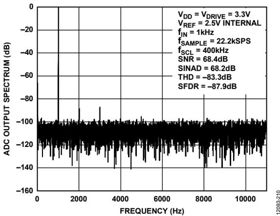
Figure 12. 10 kHz FFT,  $V_{DD} = 3.0V$ ,  $V_{REF} = 2.5V$  Internal
