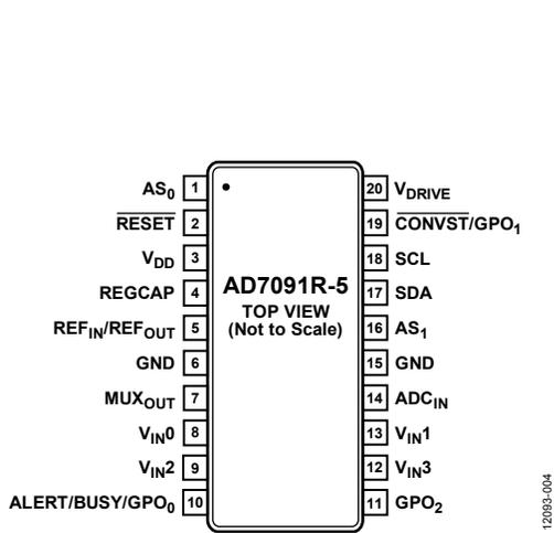
Figure 3. Pin Configuration, 20-Lead TSSOP
