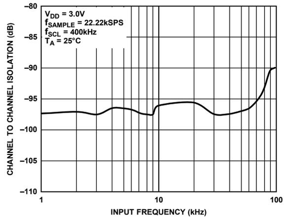
Figure 28. Channel to Channel Isolation vs. Input Frequency
