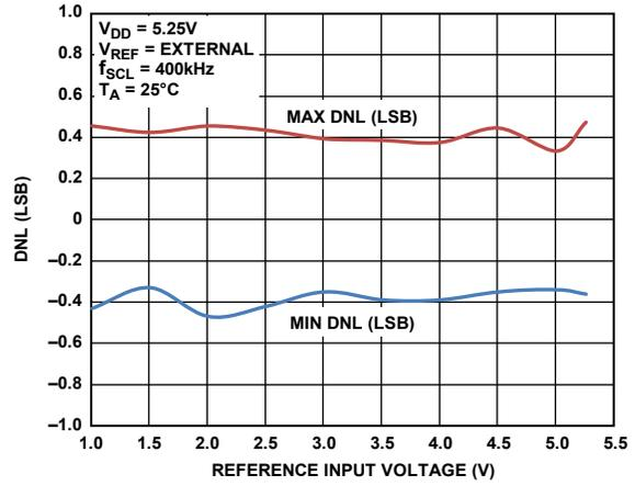
Figure 9. Minimum/Maximum DNL vs. External Reference Input Voltage
