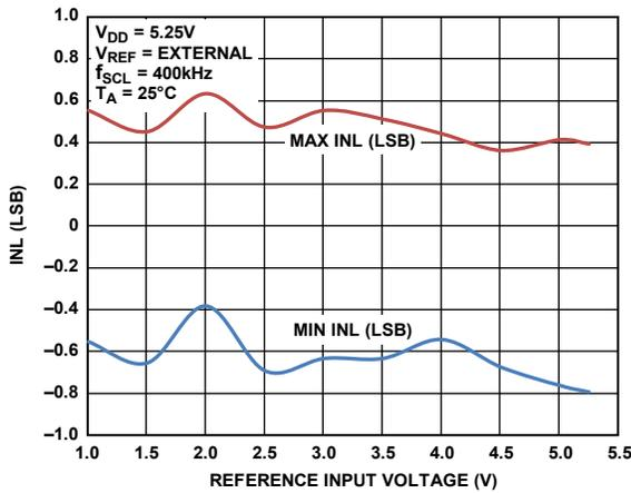
Figure 6. Minimum/Maximum INL vs. External Reference Input Voltage
