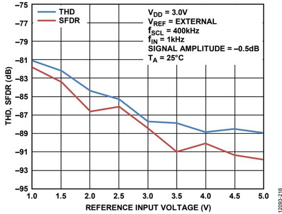
Figure 17. THD, SFDR vs. Reference Input Voltage
