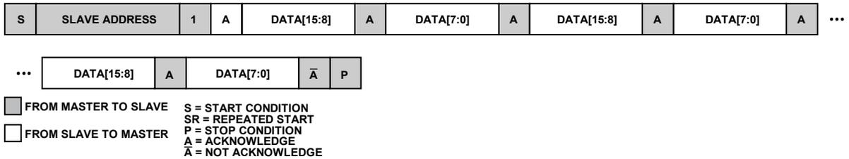
Figure 42. Reading Three Lots of Two Bytes of Data from the Conversion Result Register (Conversion Register Pointer Already Set)
