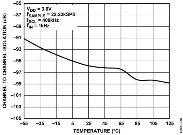
Figure 29. Channel to Channel Isolation vs. Temperature
