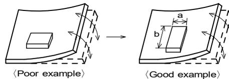
(2) Components location on PCB separation
